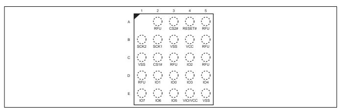
Figure 27 Dual-Quad 24-ball BGA, 5 x 5 ball footprint (ZSA024), top view
