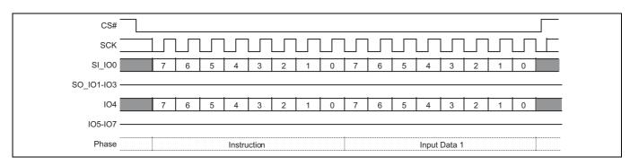
Figure 49 AutoBoot Register Write (ABWR) command
