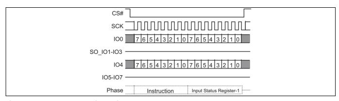
Figure 41 Dual-Quad Write Registers
