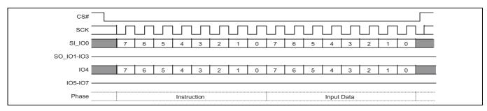
Figure 39 Bank Register Write (BRWR 17h) command
