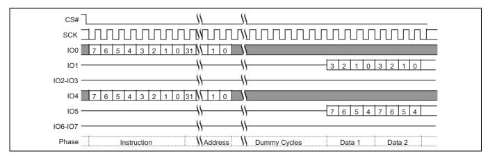
Figure 54 Dual-Quad SPI Fast Read (FAST\_READ) command sequence
