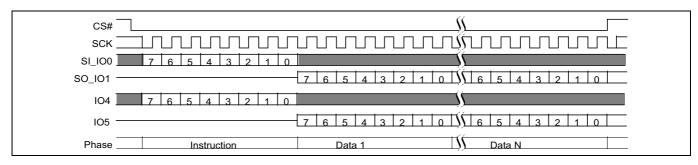
Figure 52 Dual-Quad DLP Read (DLPRD 41h) command sequence
