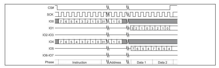
Figure 6 Dual-Quad Single bit Wide I/O command without latency
