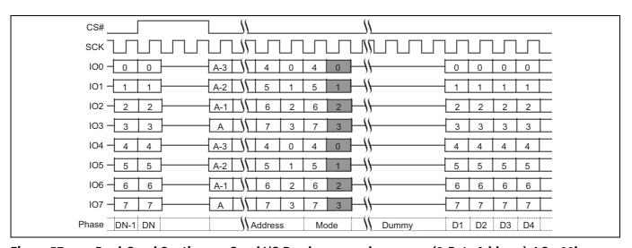
Figure 57 Dual-Quad Continuous Quad I/O Read command sequence (3-Byte Address), LC = 00b
