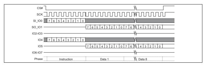
Figure 78 Password Read (PASSRD E7h) command sequence
