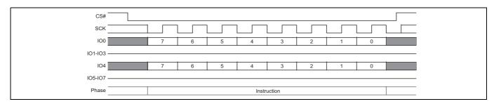
Figure 66 Dual-Quad Erase Suspend command sequence
