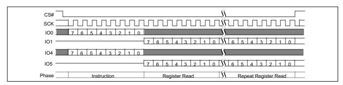
Figure 38 Read Bank Register (BRRD 16h) command
