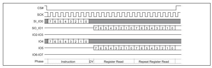
Figure 76 PPB Lock Register Read command sequence
