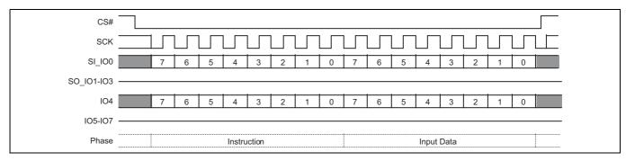
Figure 50 Program NVDLR (PNVDLR 43h) command sequence
