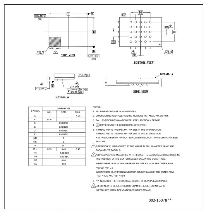
Figure 28 24-ball FBGA (8.0 × 6.0 × 1.2 mm) package outline (PG-TFBGA-24), 002-15078
