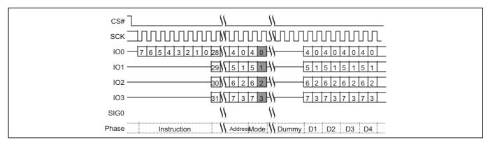
Figure 9 Dual-Quad, Quad I/O command
