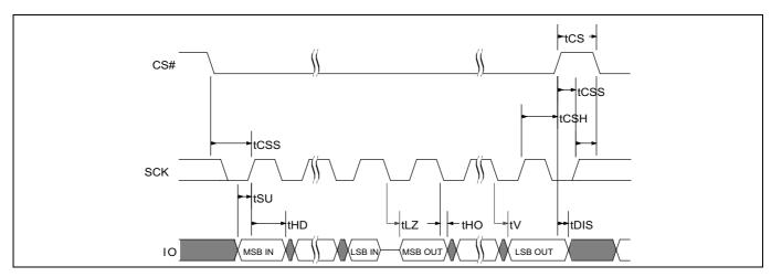
Figure 23 SPI SDR dual-quad timing
