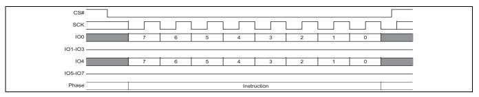
Figure 67 Dual-Quad Erase Resume command sequence
