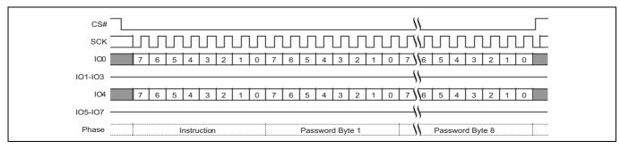
Figure 79 Password Program (PASSP E8h) command sequence
