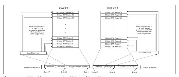
Figure 29 OTP address space — Quad SPI-1 and Quad SPI-2
