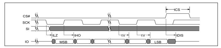
Figure 25 SPI DDR output timing
