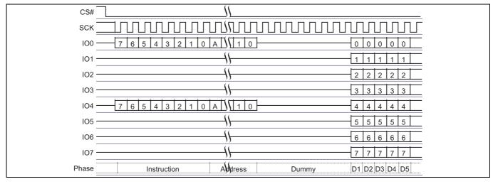
Figure 8 Dual-Quad, Quad Output Read command
