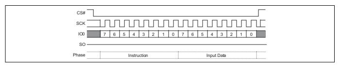
Figure 5 Dual-Quad Single bit Wide Input command
