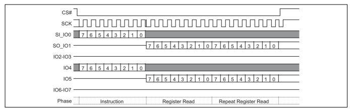
Figure 69 Dual-Quad SPI ASPRD command sequence
