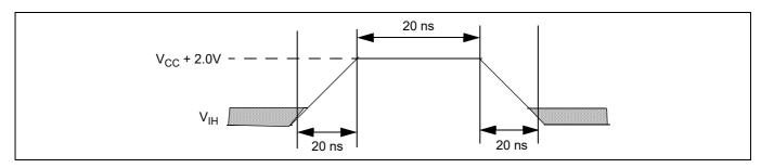
Figure 12 Maximum positive overshoot waveform
