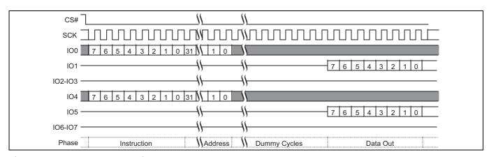
Figure 46 ECC Status Register Read command sequence
