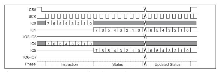
Figure 36 Dual-Quad Read Status Register 2 (RDSR2 07h) command sequence
