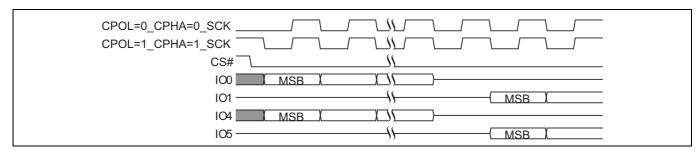
Figure 2 Dual-quad SPI SDR modes supported
