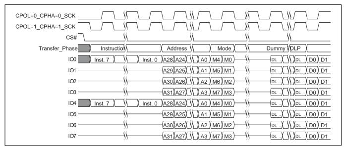
Figure 3 Dual-quad SPI DDR modes supported
