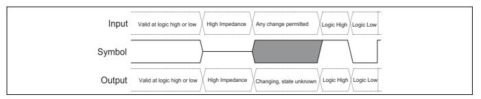
Figure 15 Waveform element meanings
