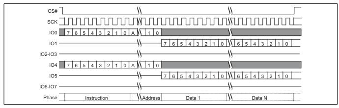
Figure 53 Dual-Quad Read command sequence (READ 03h or 13h)
