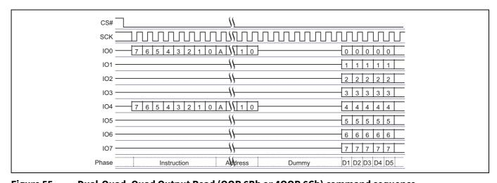
Figure 55 Dual-Quad, Quad Output Read (QOR 6Bh or 4QOR 6Ch) command sequence
