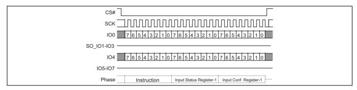
Figure 42 Dual-Quad Write Registers (WRR 01h) command sequence
