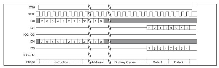
Figure 7 Dual-Quad Single bit Wide I/O command with latency
