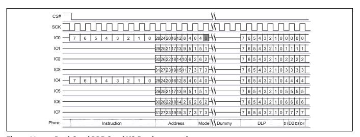
Figure 10 Dual-Quad DDR Quad I/O Read command
