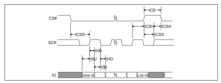
Figure 24 SPI DDR input timing
