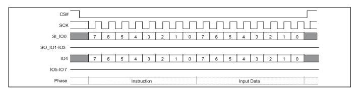
Figure 51 Write VDLR (WVDLR 4Ah) command sequence
