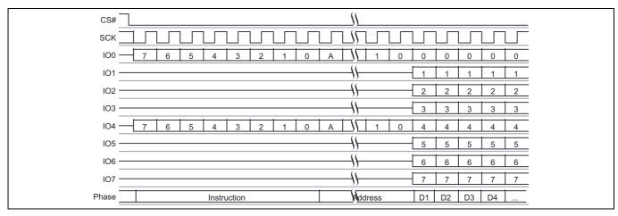
Figure 61 Dual-Quad, Quad Page Program command sequence
