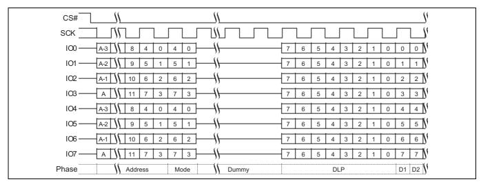
Figure 59 Dual-Quad Continuous DDR Quad I/O Read Subsequent Access
