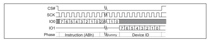
Figure 33 Read Electronic Signature (RES ABh) command sequence
