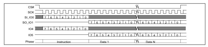
Figure 48 AutoBoot Register Read (ABRD 14h) command
