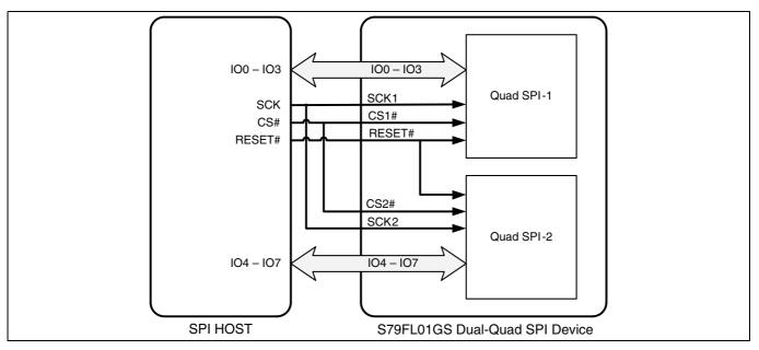
Figure 1 SPI host and S79FL01GS dual-quad SPI device with dual CS# and SCK balls in the 24-ball BGA package (5x5 ball configuration)
