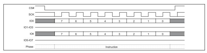
Figure 44 Dual-Quad Write Disable (WRDI 04h) command sequence
