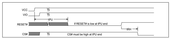
Figure 18 Reset LOW at the end of POR
