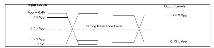
Figure 16 Input, output, and timing reference levels
