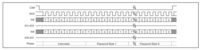
Figure 80 Password Unlock (PASSU E9h) command sequence
