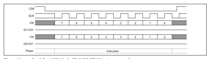
Figure 82 Dual-Quad SPI Mode Bit (MBR FFh) Reset command sequence
