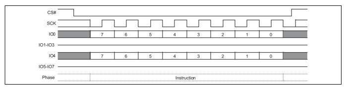
Figure 43 Dual-Quad Write Enable (WREN 06h) command sequence
