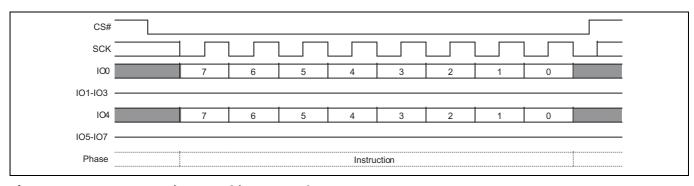
Figure 75 PPB Erase (PPBE E4h) command sequence
