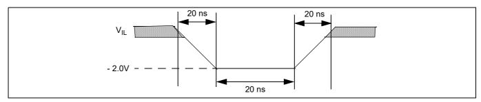
Figure 11 Maximum negative overshoot waveform
