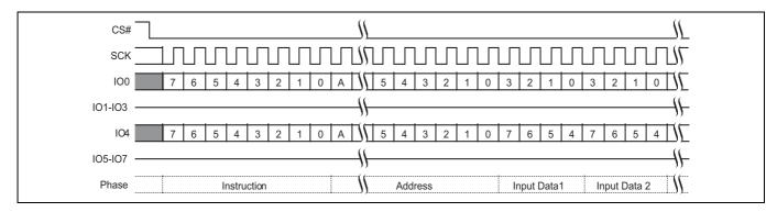
Figure 72 DYBWR (E1h) command sequence
