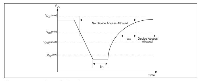
Figure 14 Power-down and voltage drop
