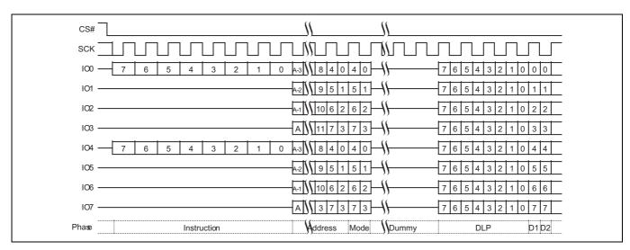
Figure 58 Dual-Quad SPI DDR Quad I/O Read Initial Access
