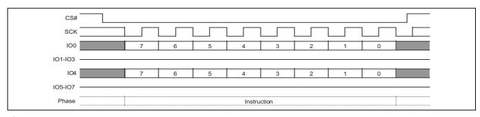
Figure 65 Bulk Erase command sequence
