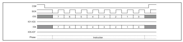
Figure 45 Dual-Quad Clear Status Register (CLSR 30h) command sequence
