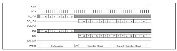
Figure 73 PPBRD (E2h) command sequence
