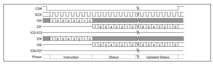
Figure 35 Dual-Quad Read Status Register 1 (RDSR1 05h) command sequence
