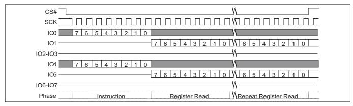
Figure 37 Dual-Quad Read Configuration Register (RDCR 35h) command sequence
