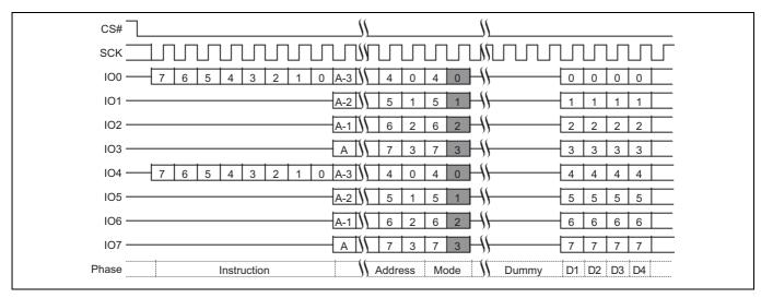
Figure 56 Dual-Quad I/O Read command sequence (3-Byte Address, EBh [ExtAdd = 0], LC = 00b)
