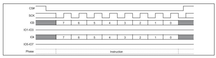
Figure 81 Dual-Quad Software Reset (RESET F0h) command sequence
