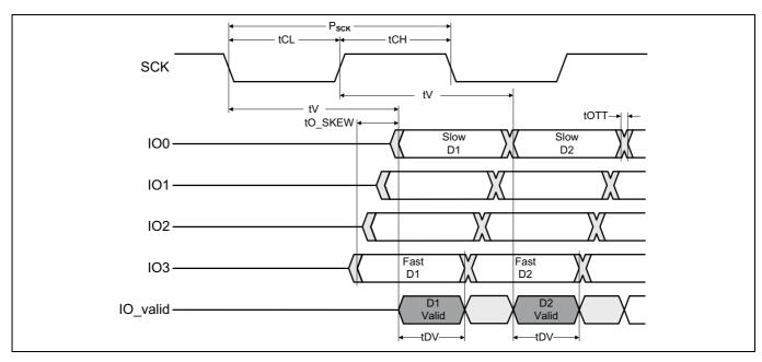
Figure 26 **SPI DDR data valid window**
