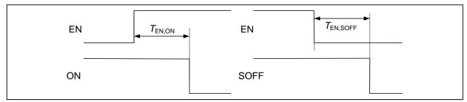
Figure 8 Timing of EN turn-on and shut down propagation delay
