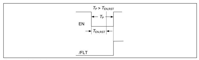
Figure 12 Timing for fault reset at terminal EN
