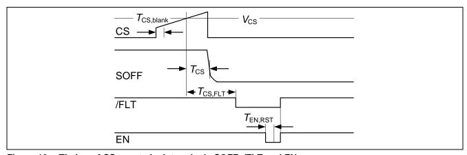
Figure 13 Timing of CS events incl. terminals SOFF, /FLT and EN
