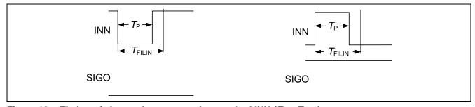
Figure 10 Timing of short pulse suppression terminal INN ( $T_P < T_{FILIN}$ )
