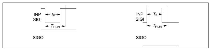
Figure 9 Timing of short pulse suppression terminal INP and SIGI ( $T_P < T_{FILIN}$ )
