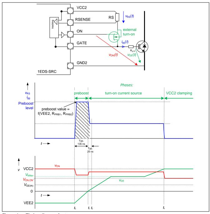
Figure 4 Timing diagram for turn-on
