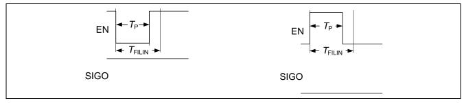
Figure 11 Timing of short pulse suppression terminal EN ( $T_P < T_{FILIN}$ )
