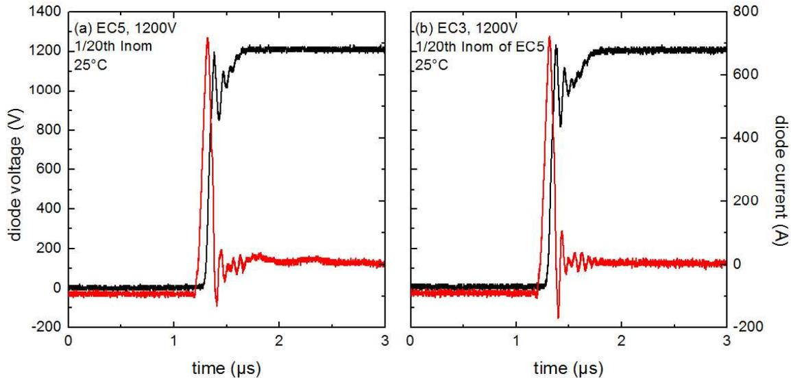
Fig. 6: Comparison of the turn-off of the 5<sup>th</sup> gen. emitter controlled diode (a) and the 3<sup>rd</sup> gen. emitter controlled diode (b) in a PrimePACK™ prototype module measured at 1/20<sup>th</sup> of the nominal current and  $T_{vj} = 25^{\circ}\text{C}$ . Red curves represent the diode current, black curves the diode voltage. Voltage and current are displayed at the same scale for (a) and (b).
