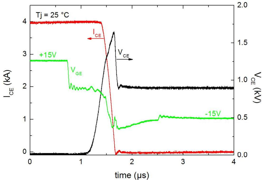
Fig. 4: Turn-off curve of a PrimePACK™ prototype module equipped with the new IGBT5 at 4000 A, more than twice the nominal current (1800 A),  $T_j = 25\text{ }^\circ\text{C}$  and an external gate resistor of 0.52  $\Omega$ . Red curves represent the collector emitter current, green and black curves represent the gate-emitter and collector-emitter voltage, respectively.
