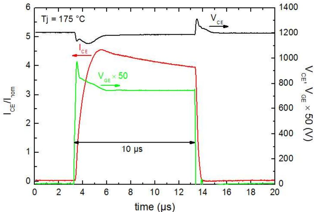
Fig. 3: Waveforms of a short circuit pulse measured on a single 1700V IGBT5 mounted on a direct copper bonded substrate using .XT technology. The collector emitter current ( $I_{CE}$ ) and the collector emitter voltage ( $V_{CE}$ ) are shown as red and black solid curves, respectively. The gate voltage (+15 V on-state) is shown as green solid curve. The DC-link voltage was 1200 V, the initial junction temperature was 175 °C, and the short circuit pulse length was 10  $\mu$ s.
