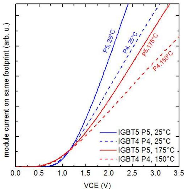
Fig. 2: Output characteristics of the 1700V IGBT5 compared with the 1700V IGBT4 (variant for high power applications P4), recorded at 25°C (blue curves) and their respective  $T_{j,op,max}$  (red curves). Solid and dashed curves represent the IGBT5 and IGBT4, respectively. The output characteristics were measured for a positive gate voltage of  $V_{GE} = 15$  V.
