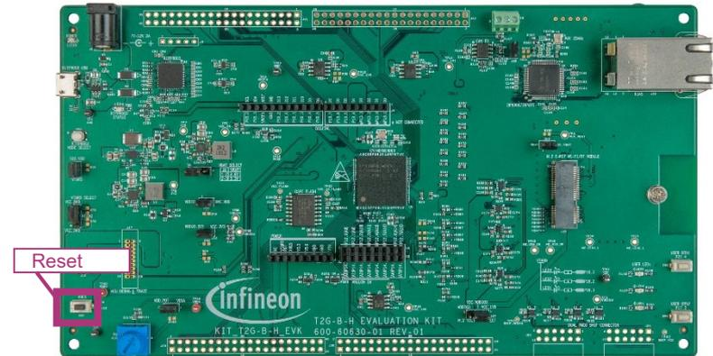
3. Press the **Reset** button to start over. The opening message appears in the terminal again.
