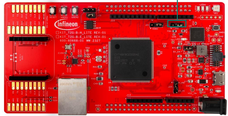
VDD current measurement jumper (J20)
