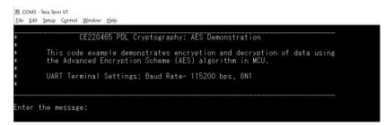
2. When you input the message for encryption, the "Enter" key is pressed, and displays the key used for encryption, encryption result, and decryption result on the terminal.
