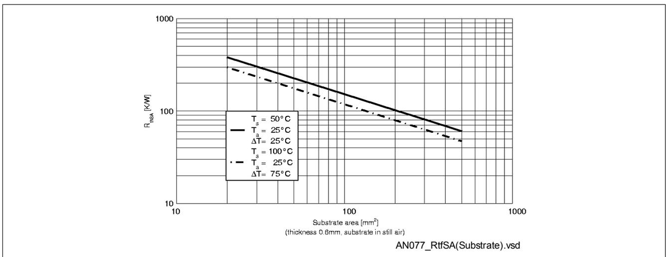
**Figure 3 Heat Dissipation from Al<sub>2</sub>O<sub>3</sub>-Substrate to Ambient Air (substrate in still air, vertical 0.6 mm thick)**
