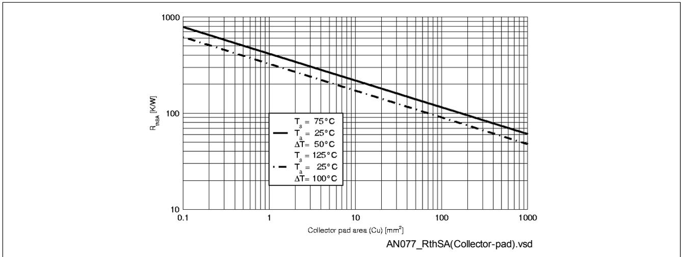
**Figure 2 Heat Dissipation from PC Board to Ambient Air (mounting pad Cu 35 μm / substrate: epoxy 1.5mm)**
