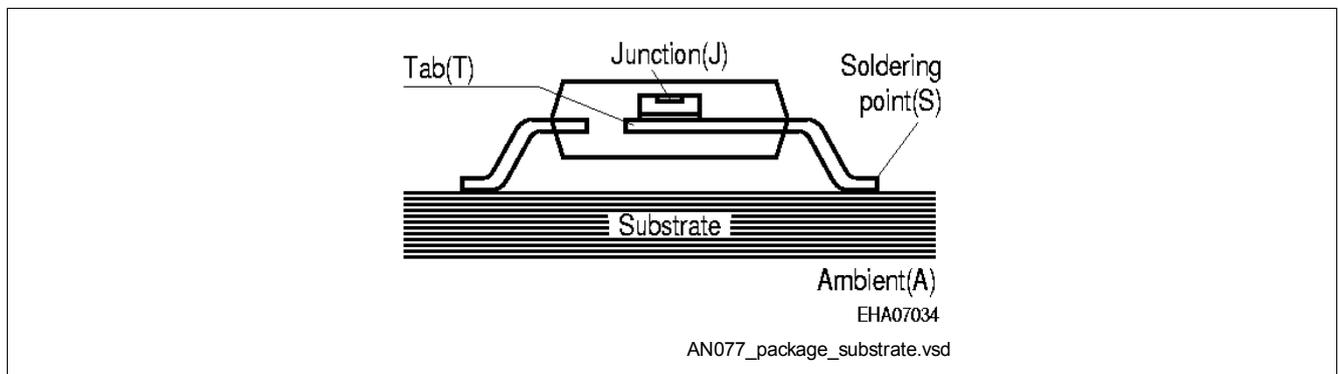
Figure 1 Package on substrate
