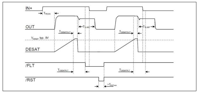
Figure 14 Two-Level Turn-Off under DESAT condition
