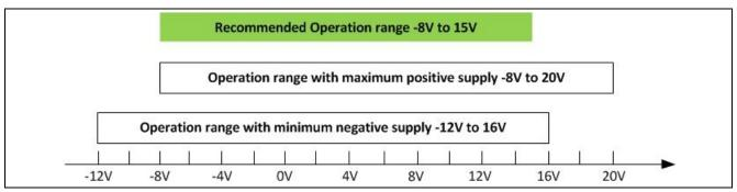
Figure 3 Supply voltage range
