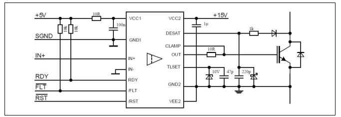
Figure 2 Typical application example unipolar supply
