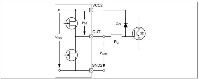
Figure 8 Rail-to-rail output
