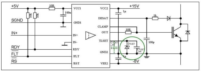
Figure 11 TLSET pin connection
