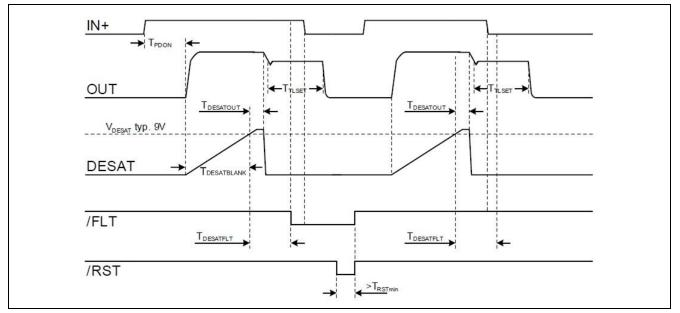
Figure 20 DESAT timing diagram
