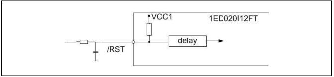
Figure 26 RESET circuit
