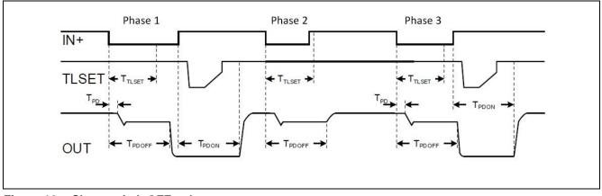
Figure 16 Short switch OFF pulses
