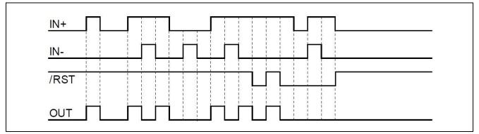
Figure 25 Principle switching behavior for RESET
