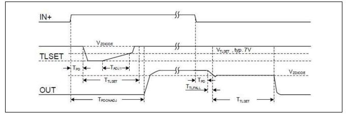
Figure 10 Two-Level Turn-Off switching behaviour
