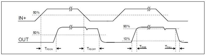
Figure 6 Propagation delay, Rise and Fall time
