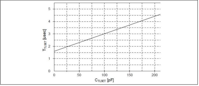
Figure 12 Typical T<sub>TLSET</sub> time over C<sub>TLSET</sub> capacitance
