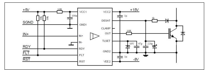
Figure 1 Typical application example bipolar supply
