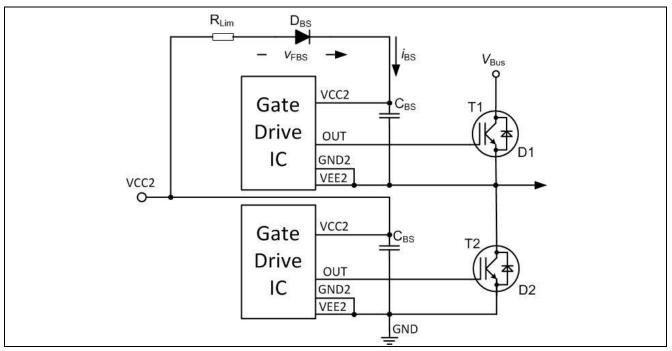
Figure 4 Bootstrap circuit for halfbridge
