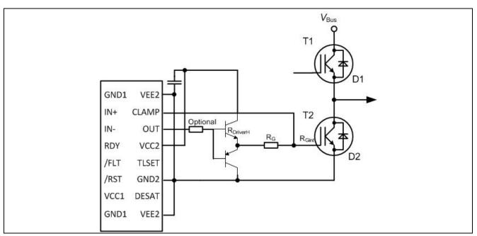
Figure 18 External booster design with clamp function and unipolar supply
