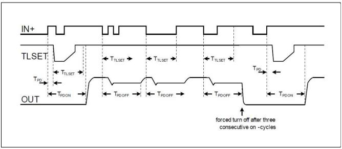
Figure 17 Short switch OFF pulses, ringing suppression
