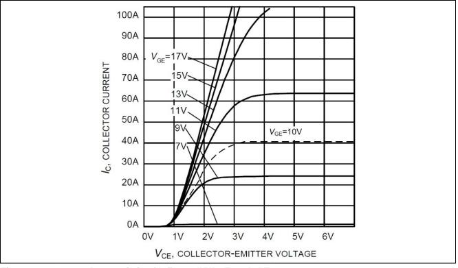
Figure 13 Output characteristic of Infineon IKW40T120 IGBT
