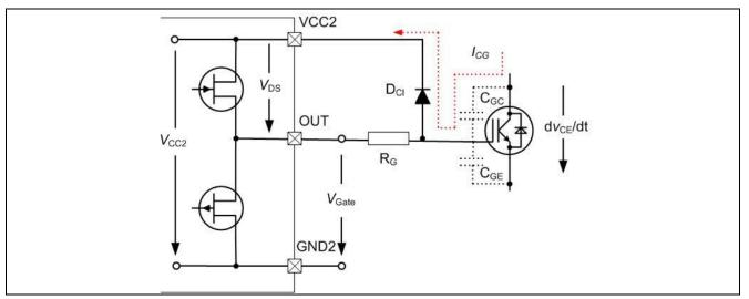
Figure 7 Short circuit clamping to VCC2, but without additional protection between OUT and CLAMP
