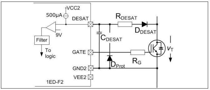
Figure 19 DESAT circuit
