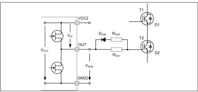
section 2.4. So it is always a trade-off inbetween. Depending on the individual parameters,  $R_{Goff}$  can be roughly half of the  $R_{Gon}$  value.
