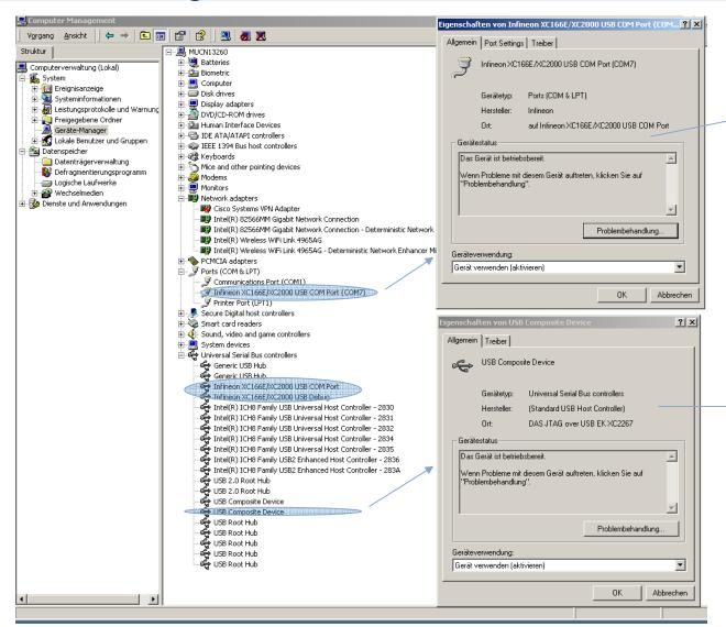
This gets identified only when COM port is used •Via the USB interface on the Easykit with FTDI chip
