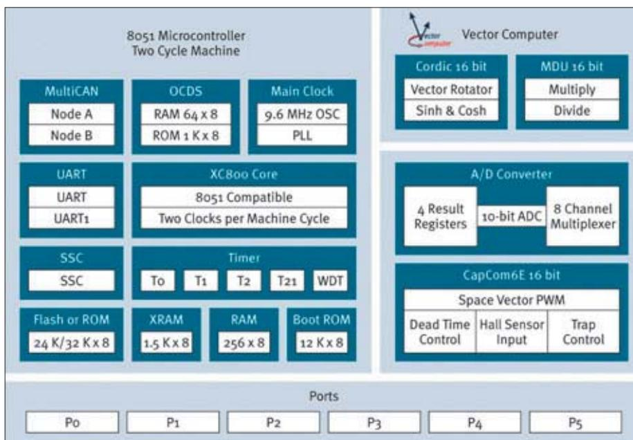
Figure 2. Block diagram of 8-bit microcontroller XC886/888 with vector computer
