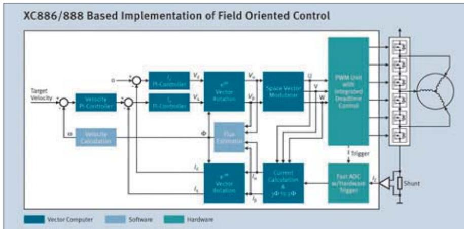
Figure 1. Sensorless Field-oriented control of PMSM motor
