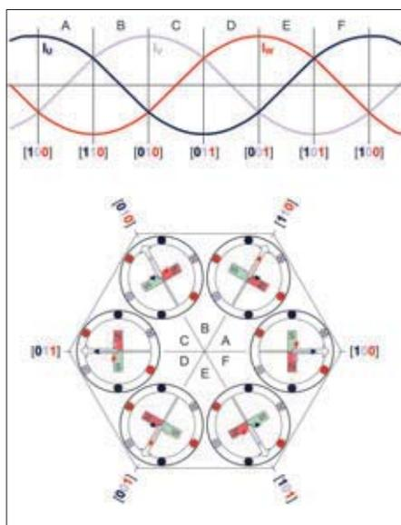
Figure 3. Sinusoidal output current and three-phase space vector, represented by a hexagon
