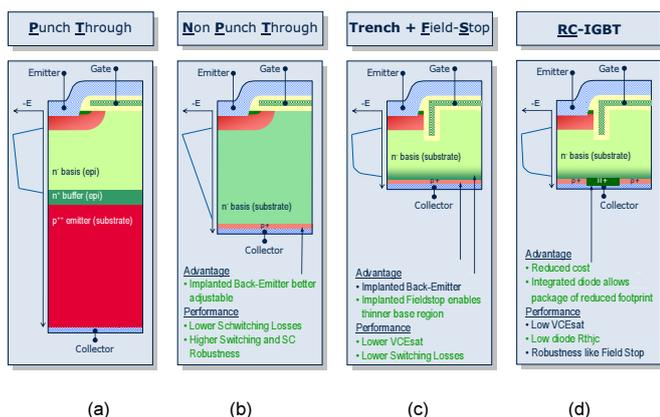
Figure 2: Vertical structures of IGBTs as a generation evolution
