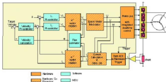
Figure 3: Block diagram of the field oriented control used in the air-conditioning system
