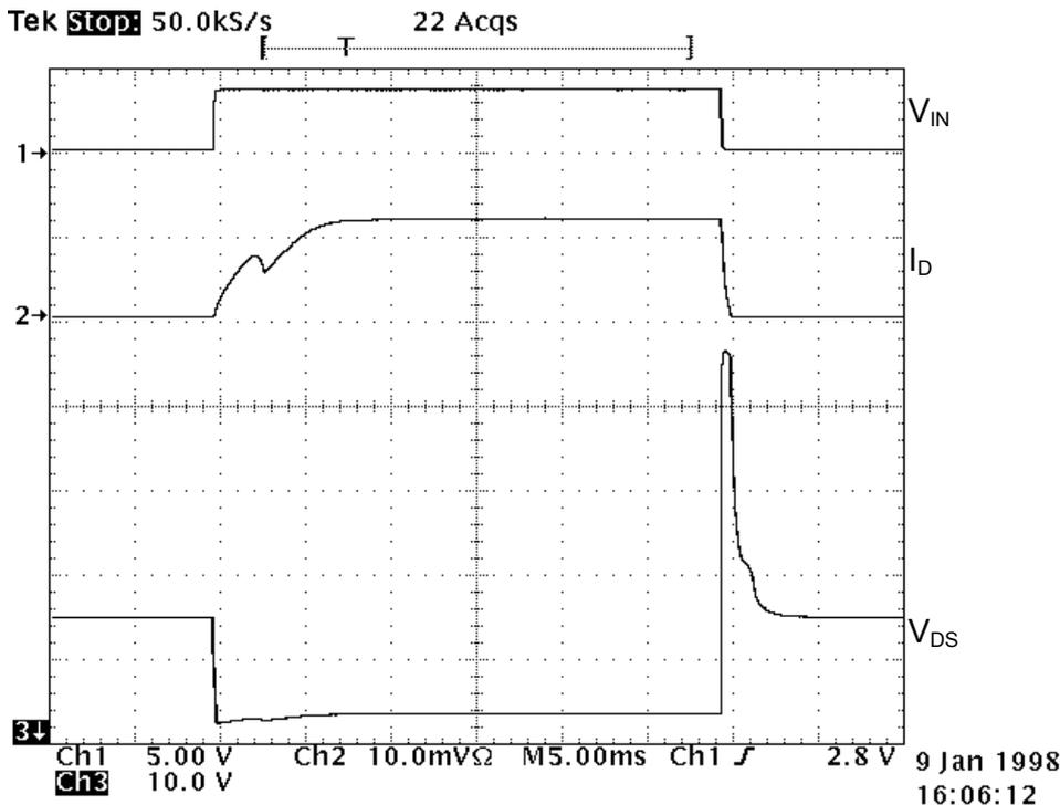
**Figure 5 Switching of a Solenoid**
