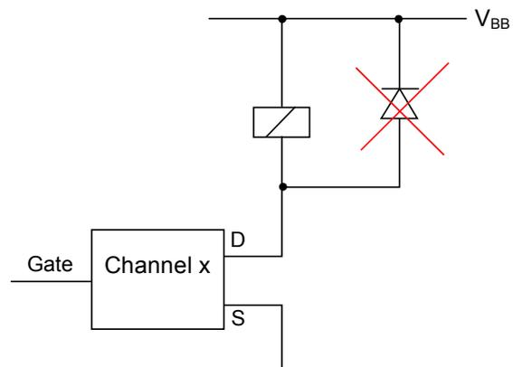
**Figure 6 Driving a relay**
