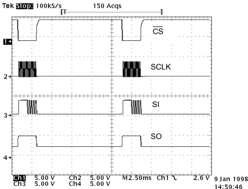
**Figure 7 Cyclic serial data transfer via SPI**
