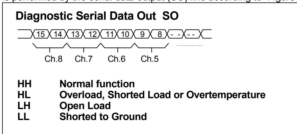
**Figure 13 Two bits per channel diagnostic feedback**
