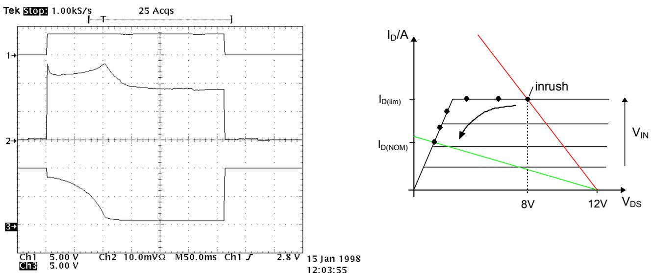
Figure 3 Switching of a Bulb
