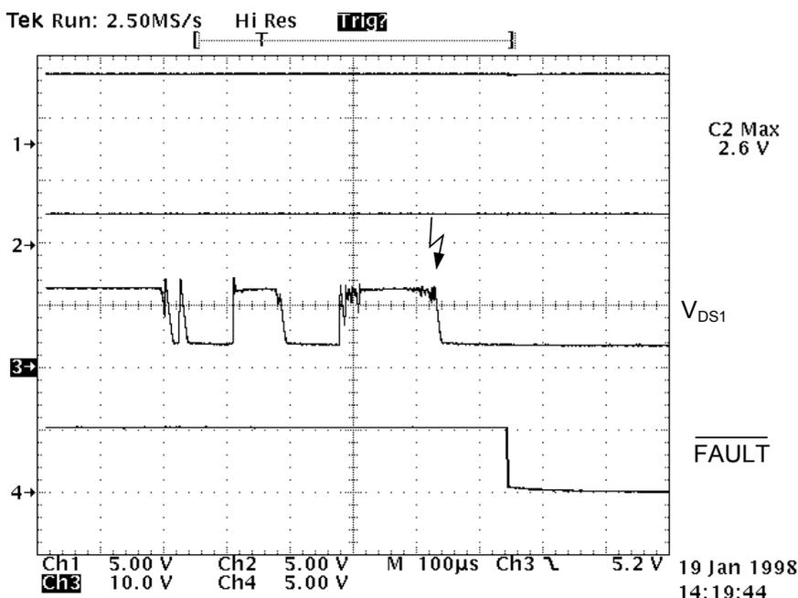
Figure 11 Fault detection via  $\overline{\text{FAULT}}$  pin
