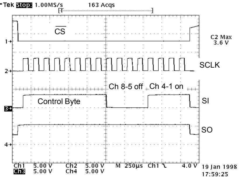
**Figure 8 Data bits 0 to 3 are programmed high to enable the parallel control for channel 1 to 4.**
