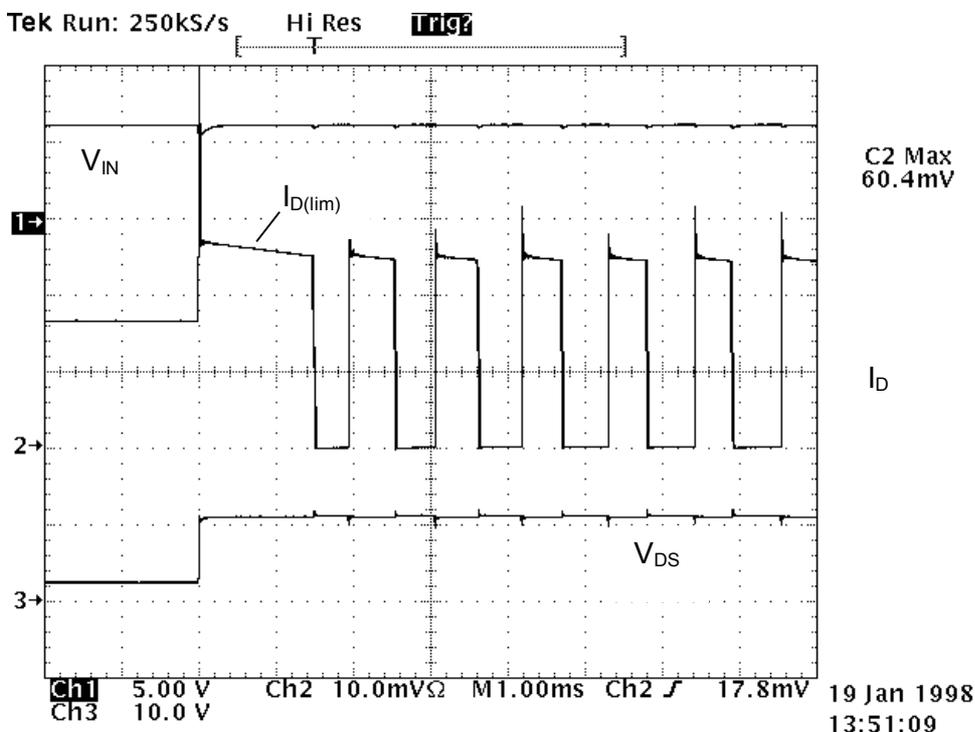
**Figure 4 Short Circuit Condition**
