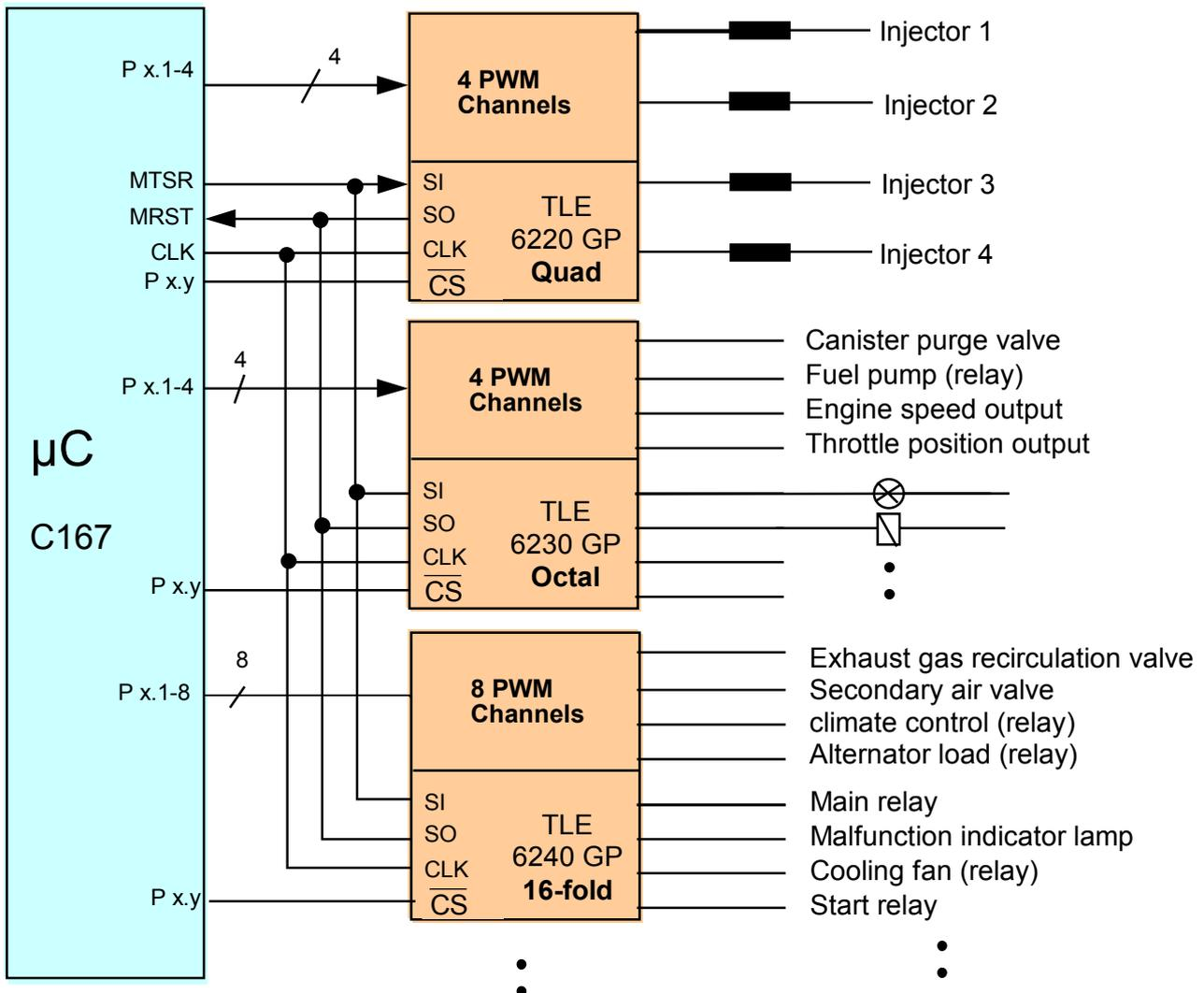
**Figure 17 Engine Management Application with the TLE 6220/6230/6240 GP**
