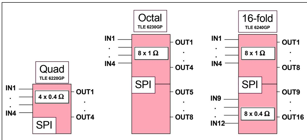
**Figure 2 Modular Concept of TLE 62x0 GP Chip Set**
