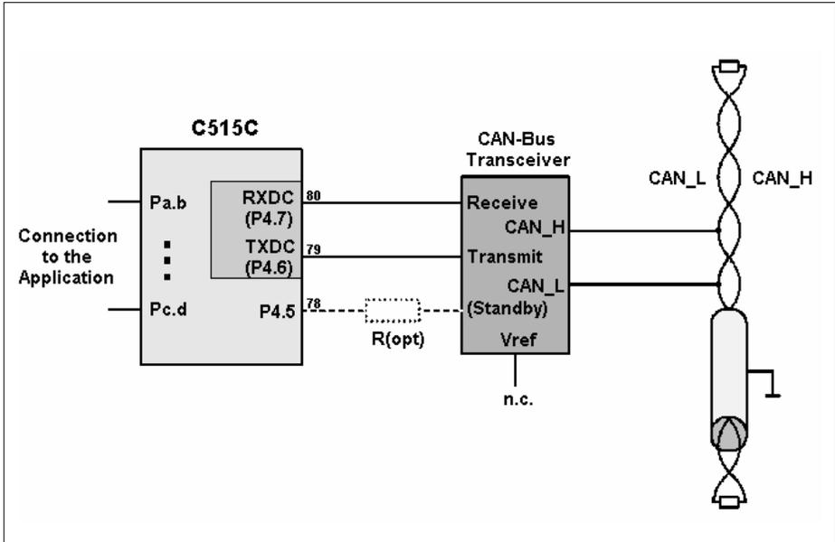
Figure 14 Connection of a C515C to CAN
