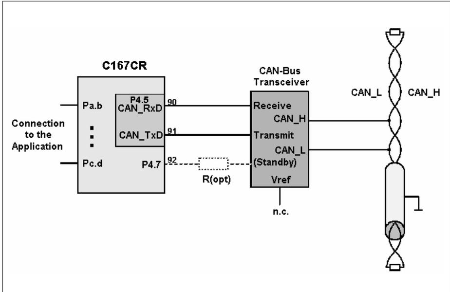
Figure 13 Connection of the C167CR to CAN
