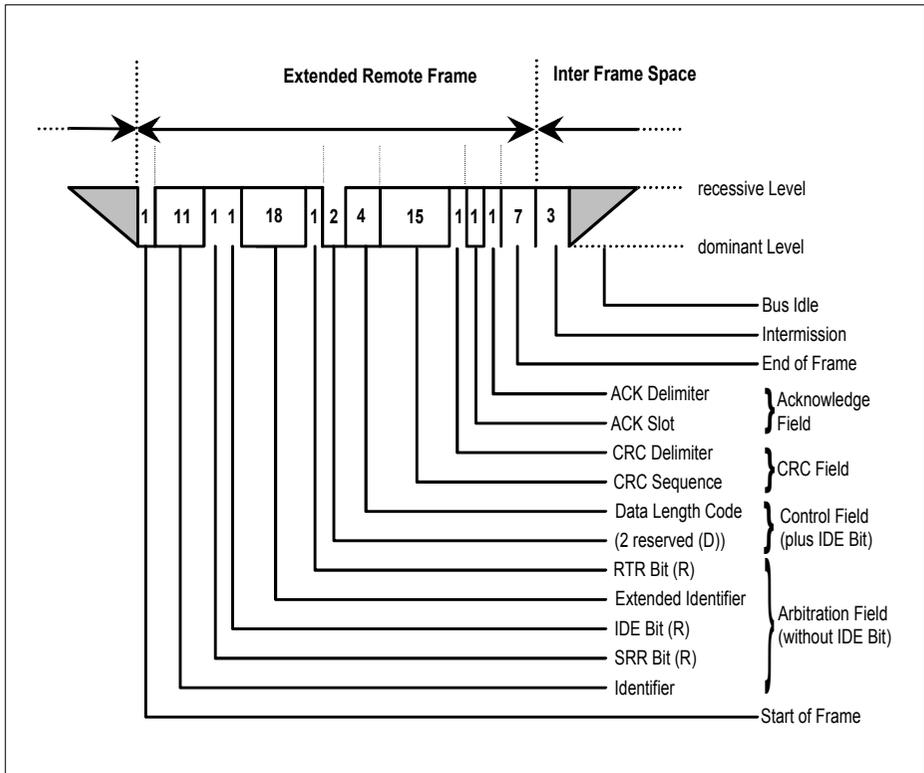
**Figure 4 Extended CAN Remote Frame**
