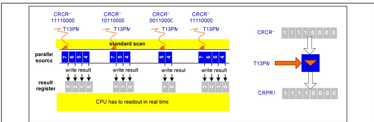
Figure 31 Timer triggered Multichannel conversion (CCU6 Timer 13 Period Match event)
