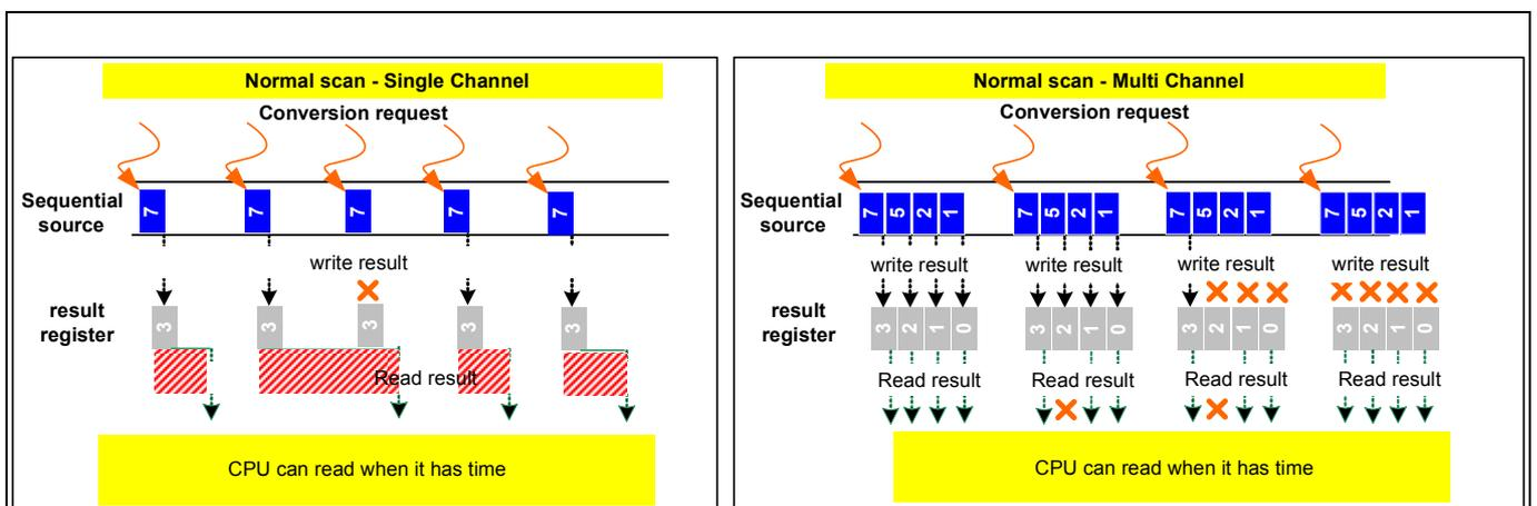
Figure 34 Sequential source single and multi channel conversion – Wait for Read mode
