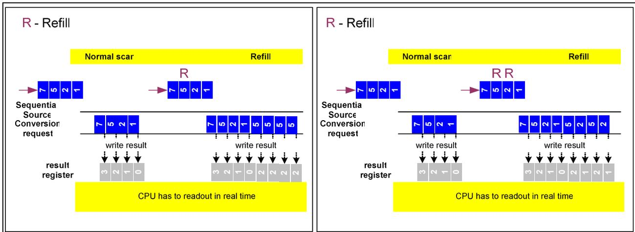
Figure 33 Sequential source single channel and multichannel conversion – Normal scan
