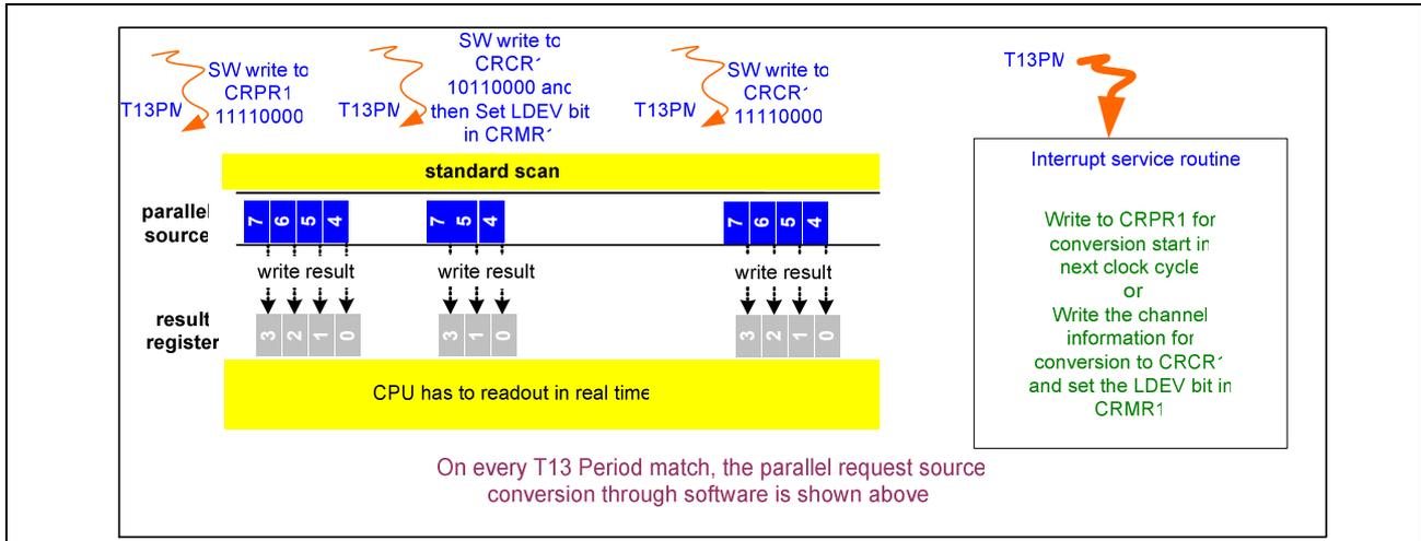
**Figure 32 Software Triggered Multichannel conversion**
