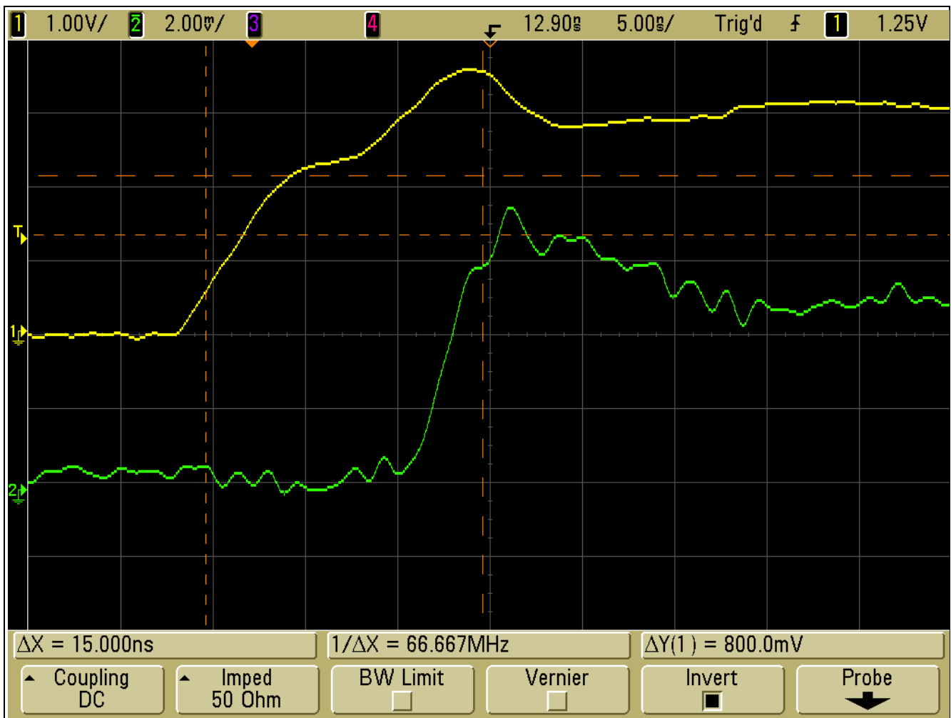
Figure 19 Oscilloscope Screen Shot, Amplifier Turn-On Time
