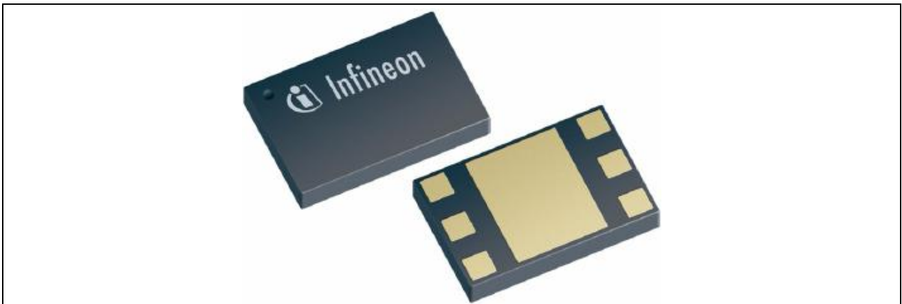
Figure 1 BGA231L7 in TSLP-7-1 Package (2 mm x 1.3 mm x 0.4 mm)
