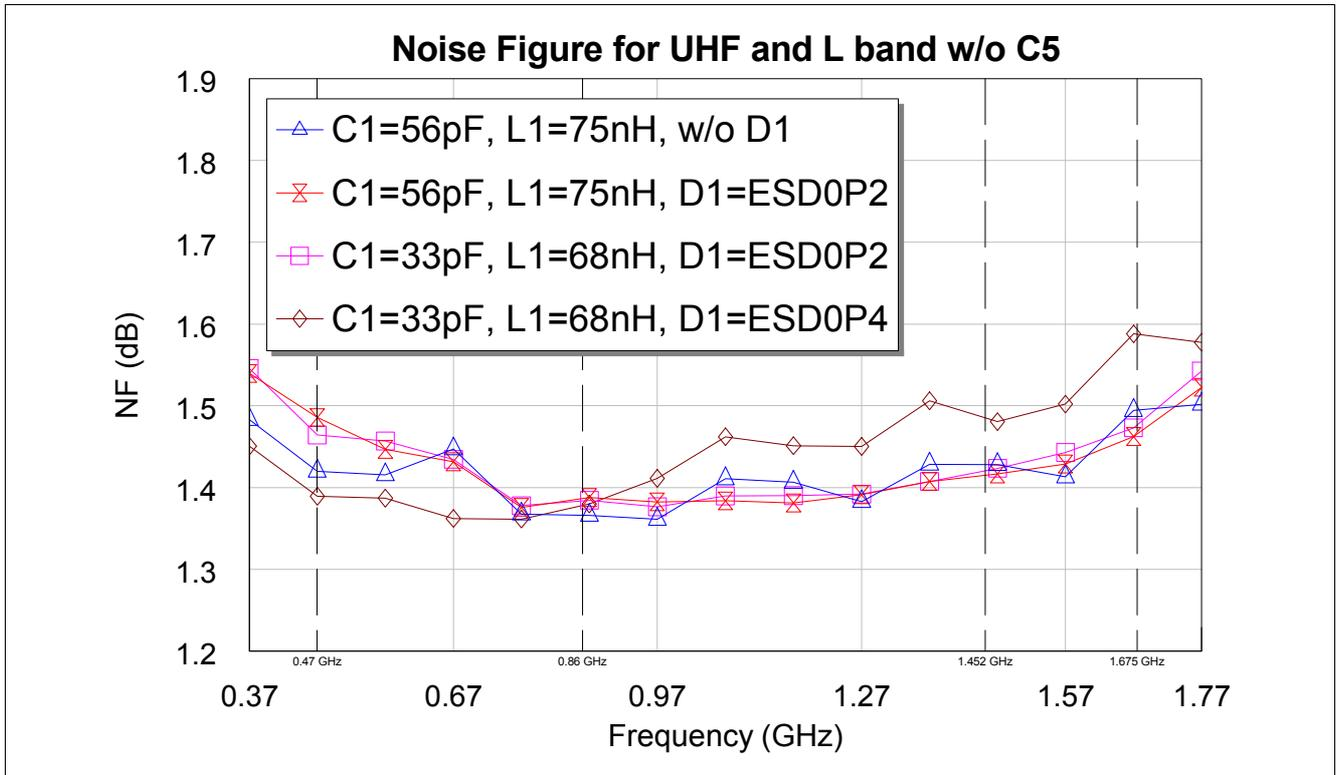
Figure 5 Noise figure in high gain mode without C5
