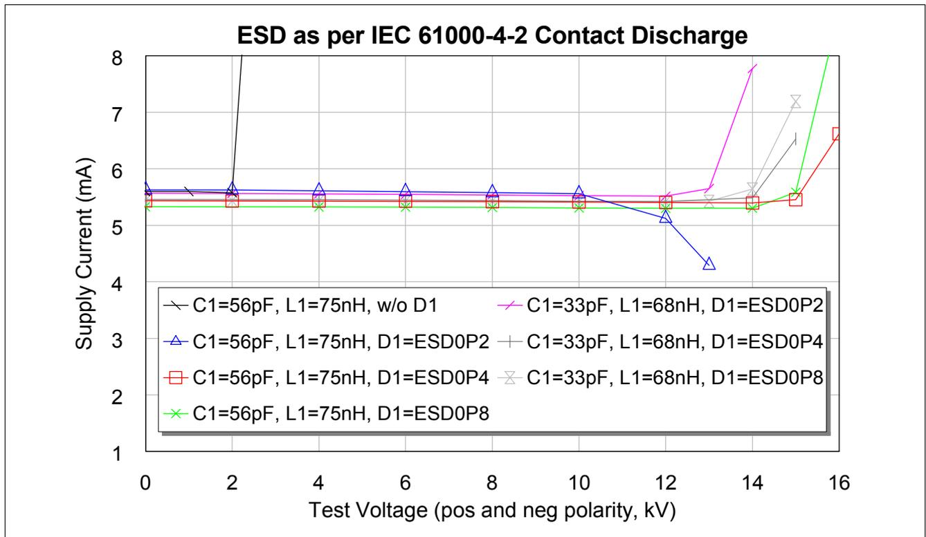
**Figure 4 ESD hardness of BGA728L7 on evaluation board as per IEC 61000-4-2 contact discharge (50 pulses per test voltage and polarity)**
