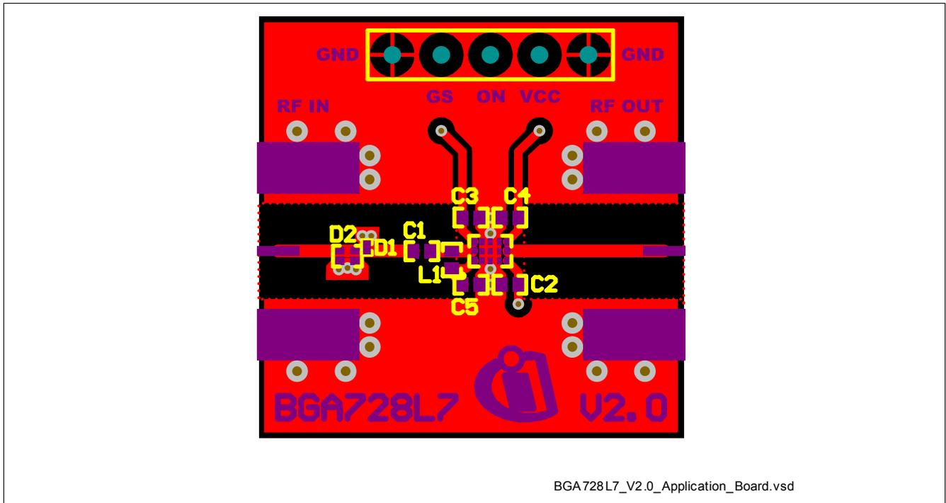
**Figure 3** Application board including ESD protection
