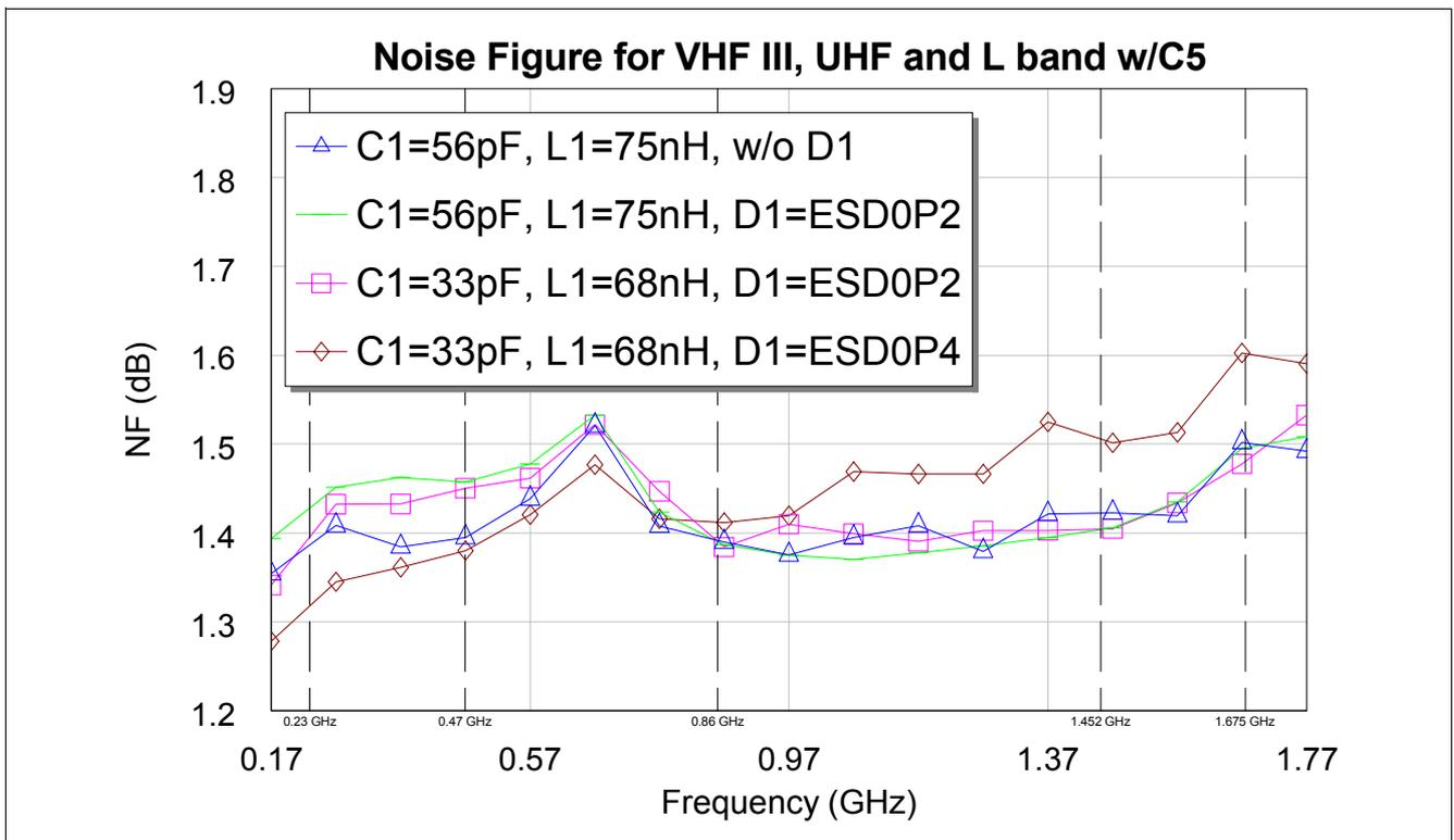
Figure 6 Noise figure in high gain mode with C5
