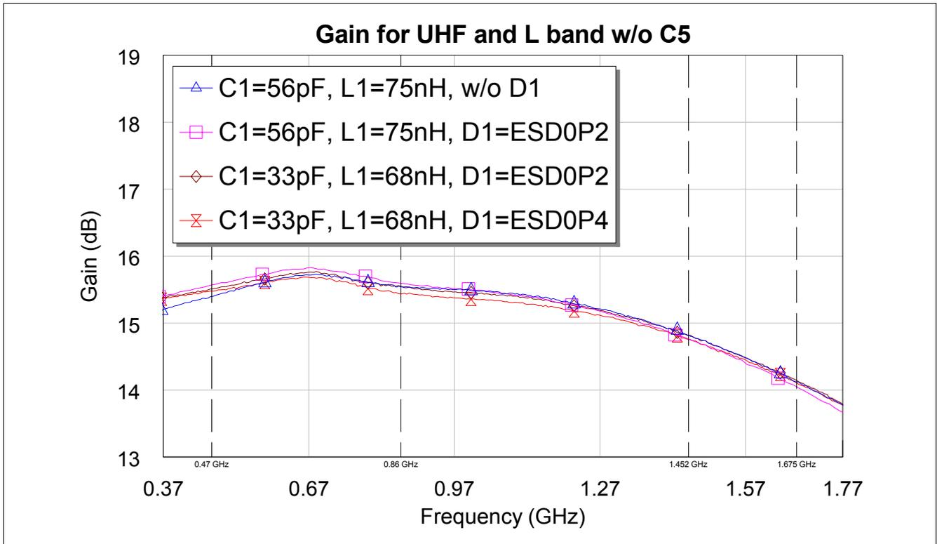
Figure 7 Power gain in high gain mode without C5
