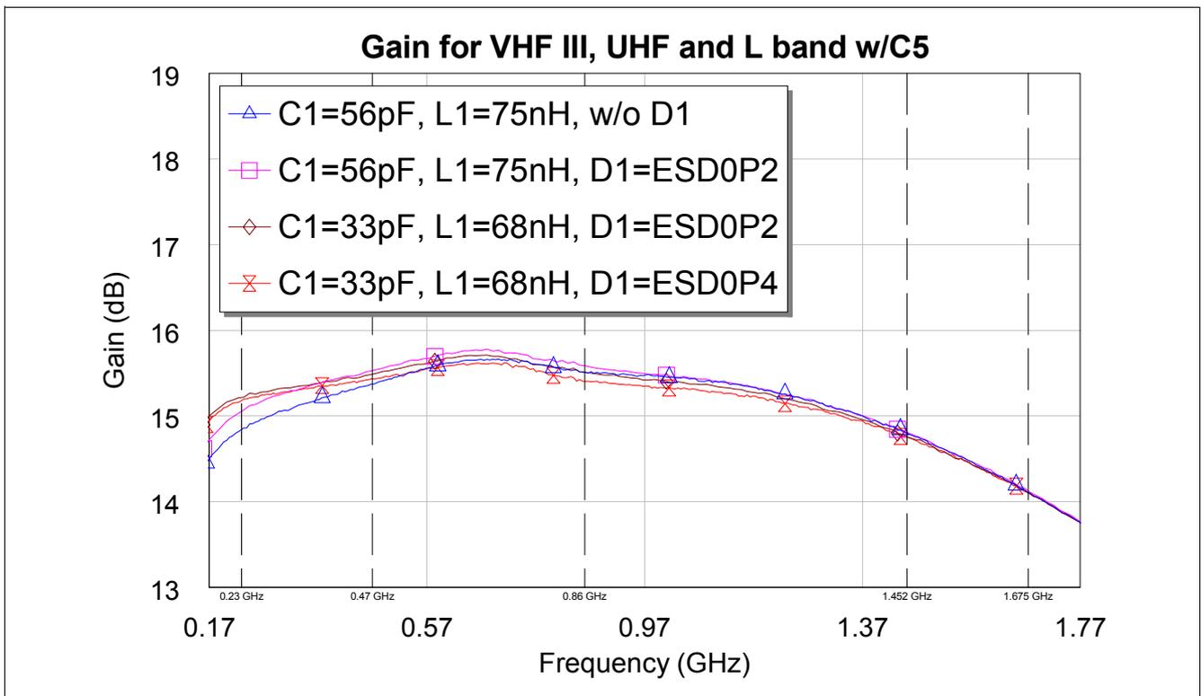
Figure 8 Power gain in high gain mode with C5
