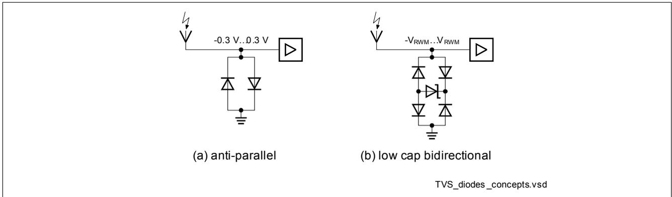
**Figure 1** Two different concepts for ESD protection of RF antennas: (a) two fast switching diodes in anti-parallel configuration, (b) a combination of four fast switching diodes and one TVS Zener diode to get a low capacitive, bidirectional TVS diode (simplified diagram)
