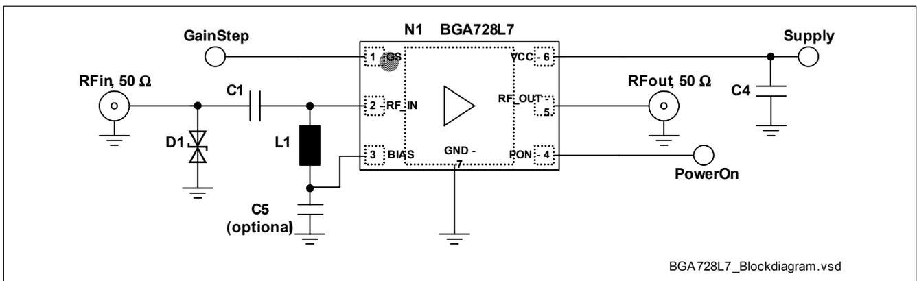
**Figure 2** Application circuit of BGA728L7
