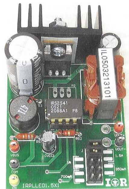
Figure 4. The IRS2540 LED converter demo board.
