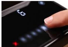
Capacitive sense slider
