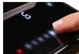
Capacitive sense slider
