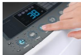
Capacitive sense buttons
