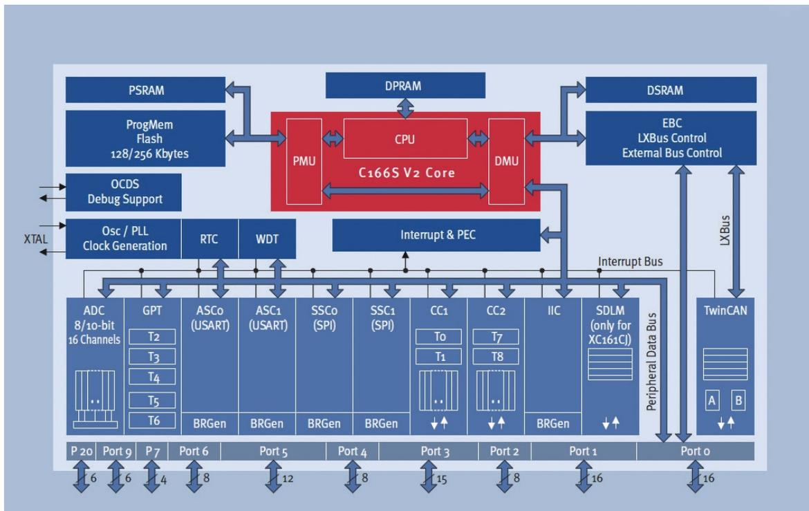
Fig. 5: Block diagram of the XC161CS high performance with 40 MHz and extensive peripherals mean that the controllers are ideally suited for numerous sensor applications such as the S300 Mini
