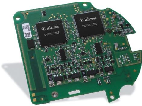
Fig. 4: Base board of the S300 Mini with the two XC161CS microcontrollers. Using the Infineon controllers saves e.g. Numerous external peripherals on the restricted board space
