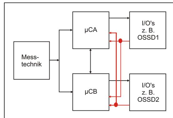
Fig. 3: Two-channel circuit design with mutual monitoring of the I/Os for high safety (SIL 2) in the S300 Mini (image: SICK)
