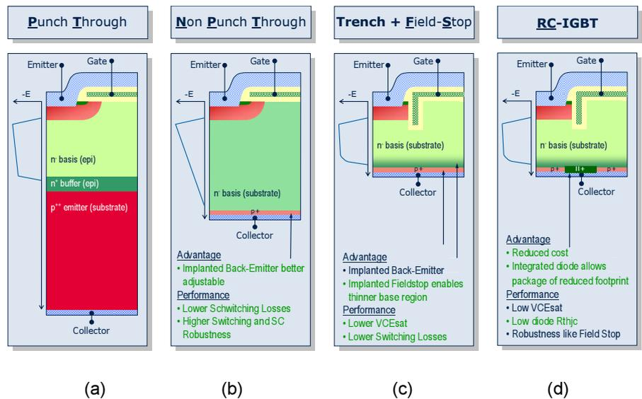
Figure 2: Vertical structures of IGBTs as a generation evolution
