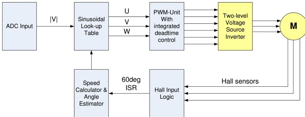
Fig 4. Control block diagram of stable operation.
