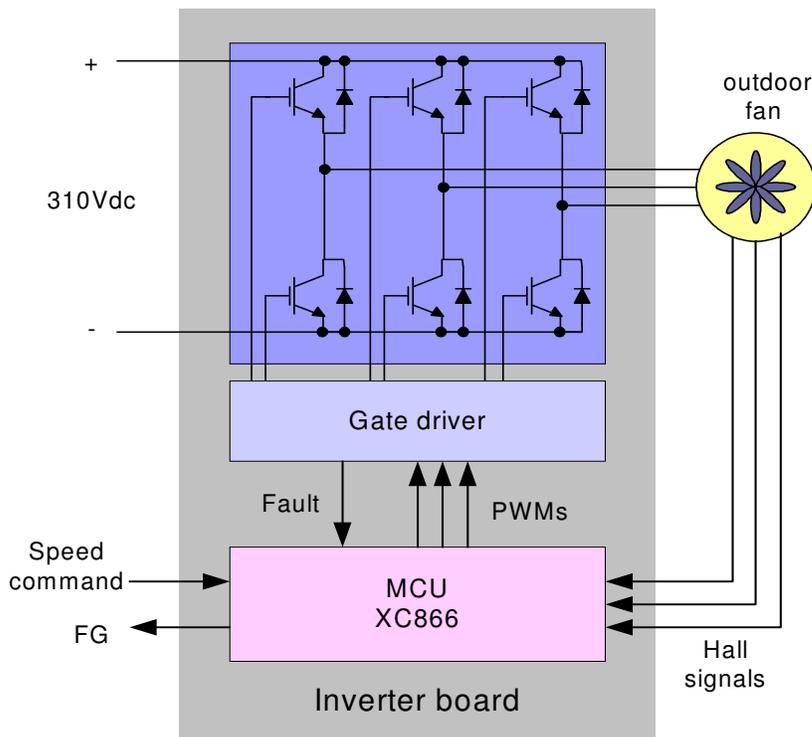
Fig 3. System block diagram of outdoor fan inverter board.
