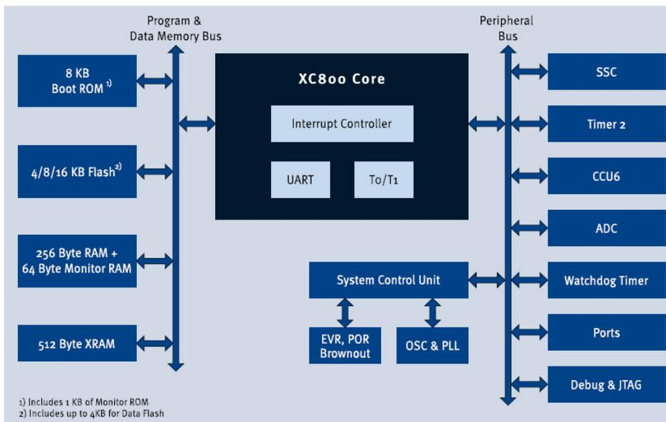
Fig 2. Block diagram of XC866 8bit micro-controller.
