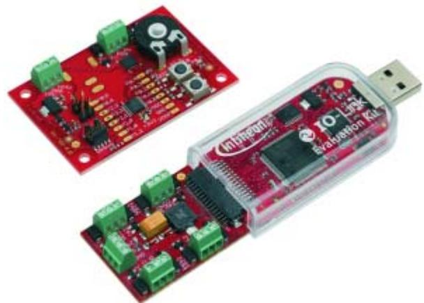
Figure 5: The IO-Link kit permits the simple evaluation of the functionality of a complete IO-Link-based master device configuration on the basis of the XE166 MCUs and XC800 devices (8 bit).
