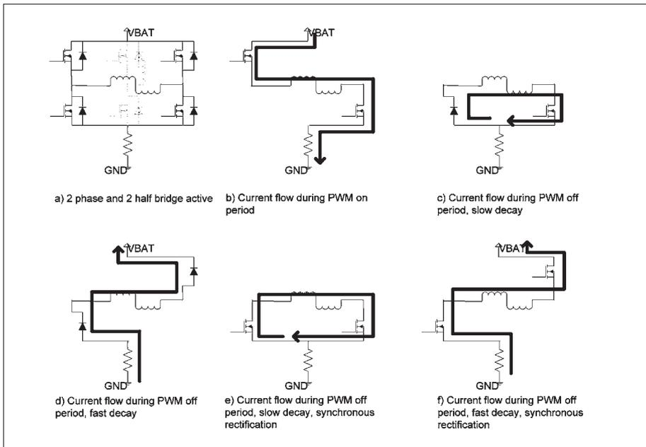
Figure 1. Pulse Width Modulation methods
