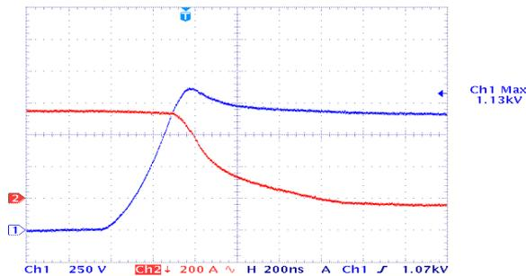
Fig. 11: IGBT turn-off at  $V_{CE}=900\text{V}$ ,  $I_C=600\text{A}$ ,  $T_{vj}=145^{\circ}\text{C}$ ,  $I_{rms}=440\text{A}$ ,  $R_G=1,6\Omega$  recorded during inverter operation at  $2,5\text{kHz}$ .
