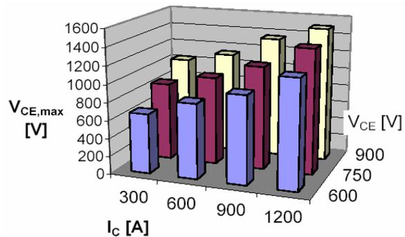
Fig. 13:  $V_{CE,max}$  for turn-off at room temperature,  $L_{\sigma}=42\text{nH}$ , no  $V_{CE}$  clamping is applied.
