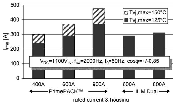
Fig. 12: usable rms current in a ModSTACK™ inverter for different 1700V IGBT modules and rated currents.
