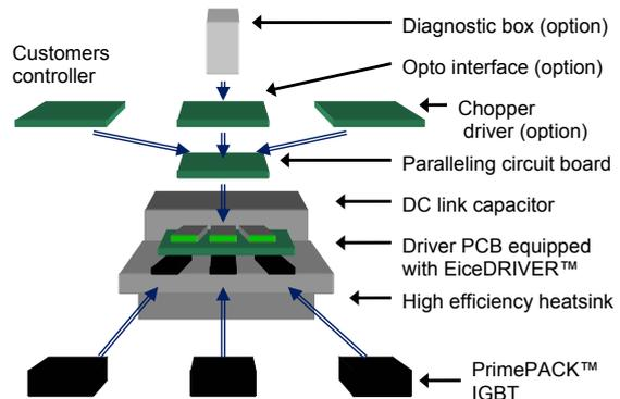
Fig. 1: Modular ModSTACK™ power unit equipped with PrimePACK™ IGBT halfbridge modules
