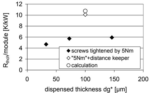
Fig. 7: Correlation between  $R_{thch}$  and grease thickness  $d_g^*$ , which is measured prior to mounting.
