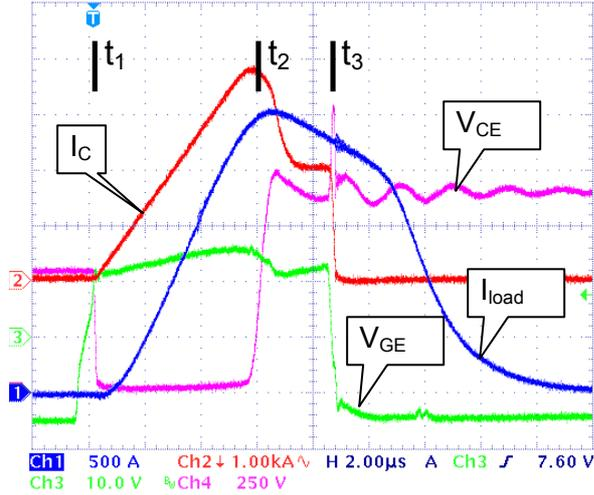
Fig. 5: Turn-off by  $V_{CEsat}$  detection after IGBT desaturation, Ch1=Load current, Ch2=IGBT collector current, Ch3=IGBT Gate voltage, Ch4=IGBT collector voltage
