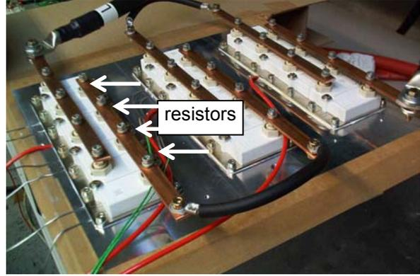
Fig. 8: Experimental setup for  $R_{thha}$  measurement. A DC current is fed into reference resistors fixed to a PrimePACK™ baseplate that is mounted on an aluminium air cooled heatsink
