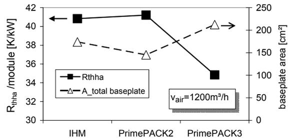
Fig. 9: Experimental  $R_{thha}$ -values for different reference-modules on an air cooled heatsink with surface=400x400mm<sup>2</sup> and height=88mm.
