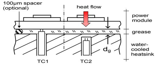
Fig. 6: Schematic cross section of measurement setup including position of thermocouples.
