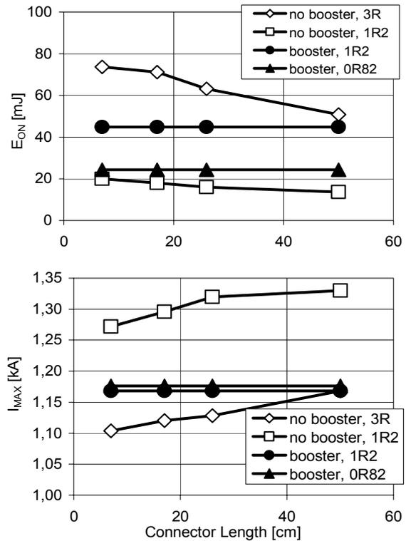
Fig. 10a/b (top/bottom): Dependence of switching parameters  $E_{on}$  (top) and  $I_{max}$  (bottom) on length of cable connecting the IGBT to the driver board for FF800R12IE4.  $U_{DC}=600V$ ,  $I_C=800A$ ,  $T_{vj}=25^\circ C$
