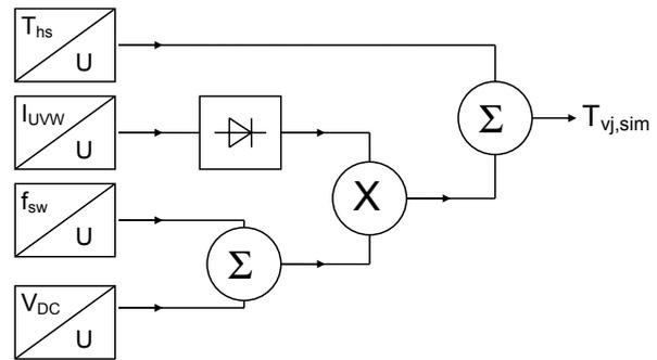
Fig. 4: logic array of the fast analogue circuit that combines  $T_{hs}$ ,  $I_{UVW}$ ,  $f_{sw}$  and  $V_{DC}$  to calculate chip temperature  $T_{vj,sim}$  by a simplified model.
