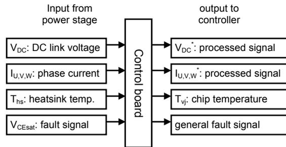
Fig. 3: flow of monitoring signals and function of control board
