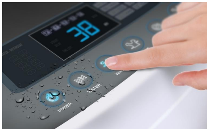
Figure 2-21 Liquid-Tolerant CapSense-Based Touch User Interface in a Washing Machine
