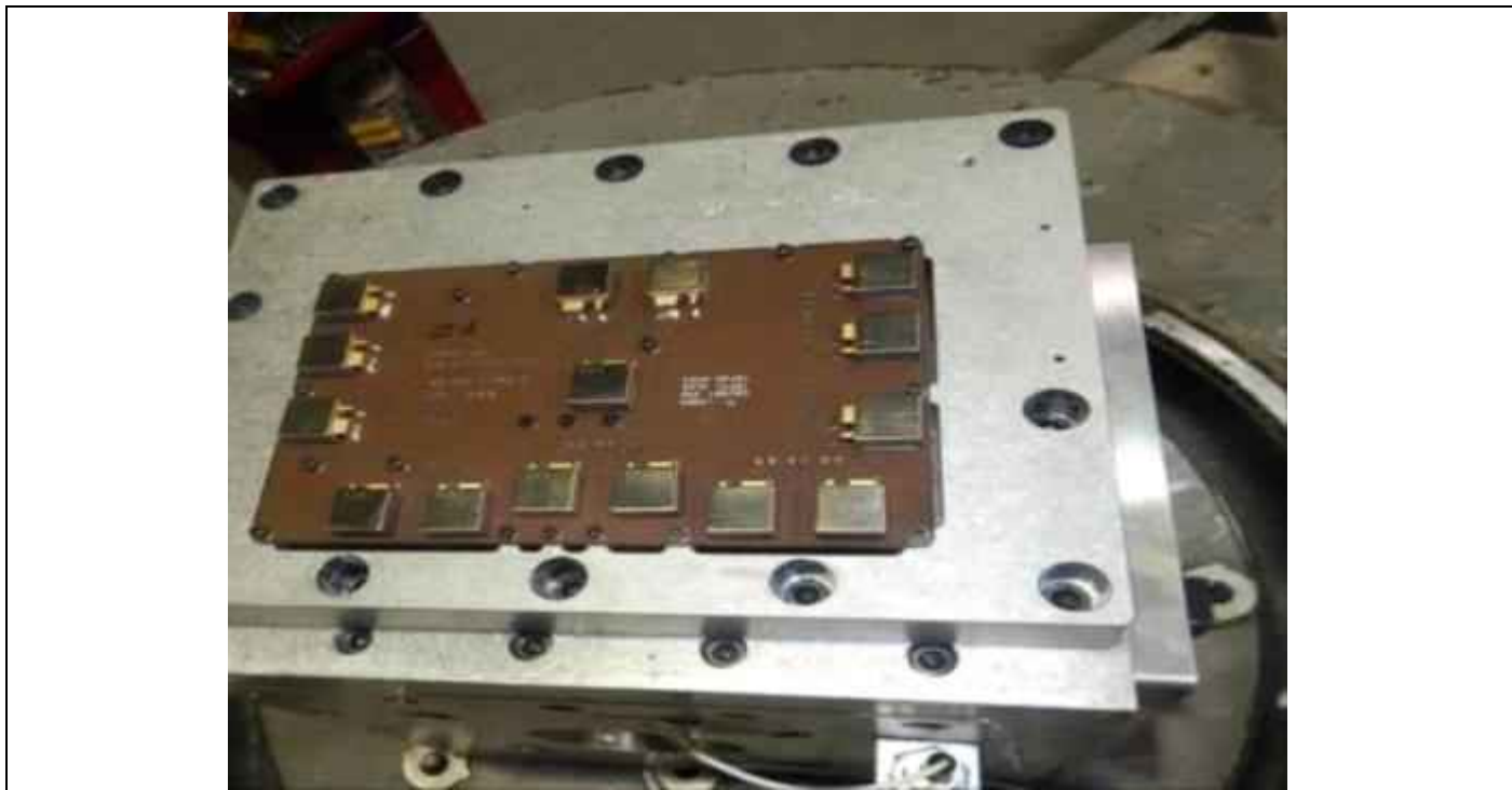
Figure 24 Z-axis random vibration setup
