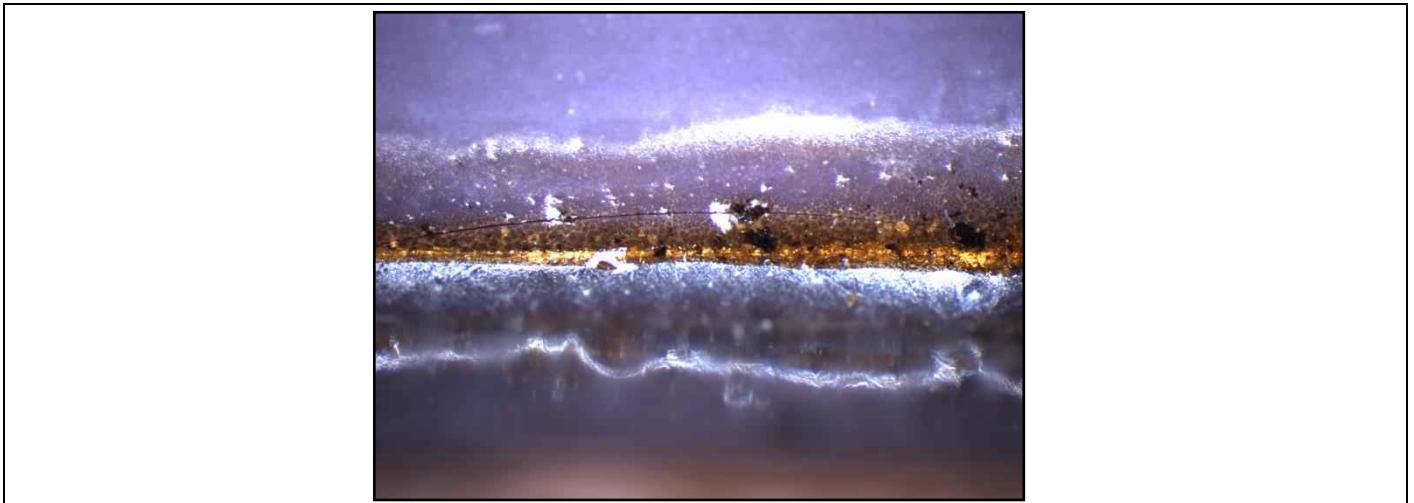
Figure 3 Stress fracture in a surface mount device on a circuit board
