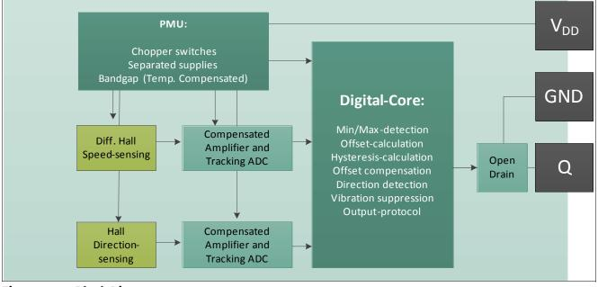
**Figure 3 Block Diagram**
