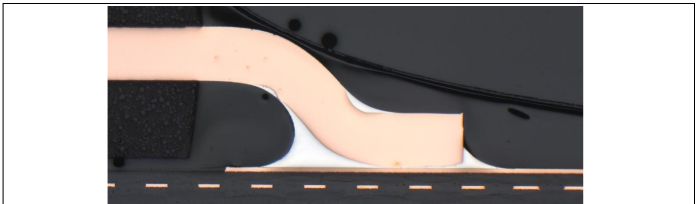
Figure 7 Cross-section of a HSOG package lead with proper solder connection to board.
