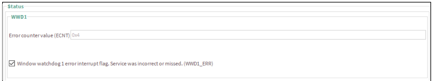
Figure 15 WWD1 error counter after 2 watchdog services were skipped
