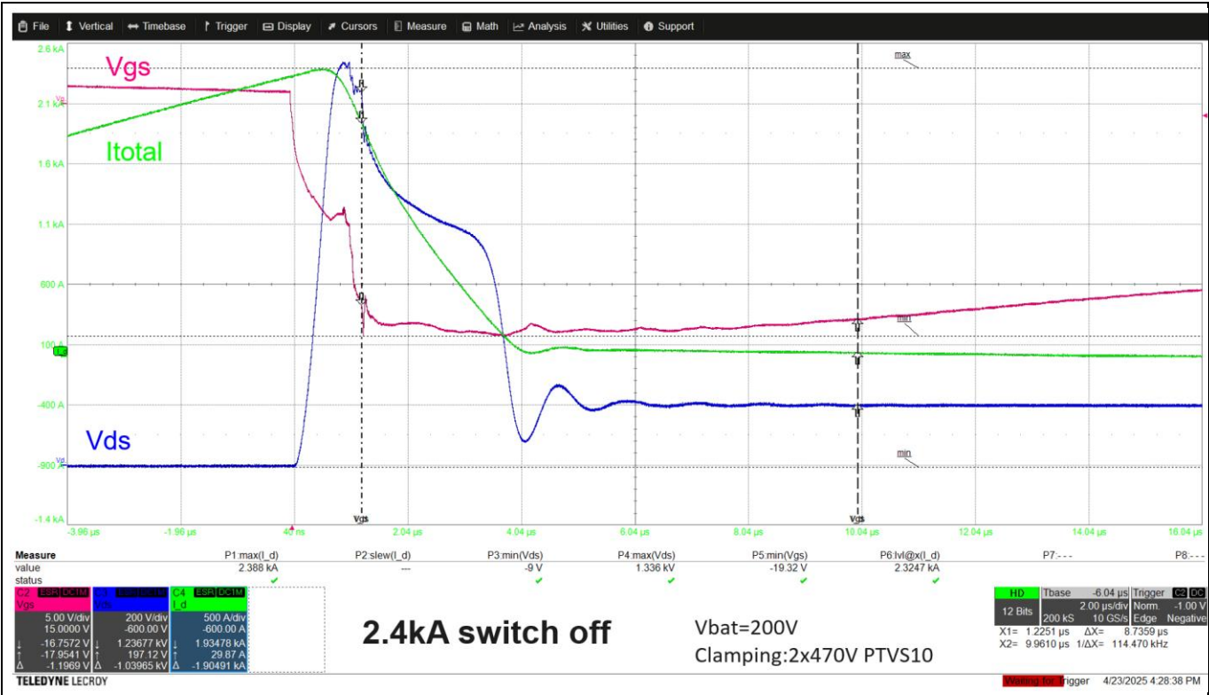
Figure 37 High-current shutdown: V bat = 200 V, I shutdown = 2.4 kA
