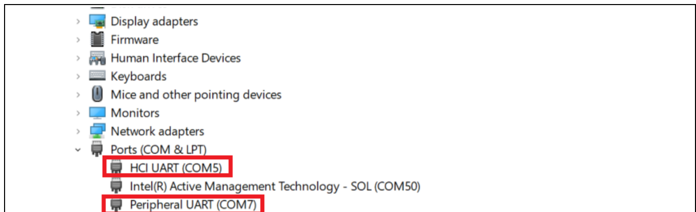
Figure 2 Virtual serial port from CYW920822M2P4XXI040
