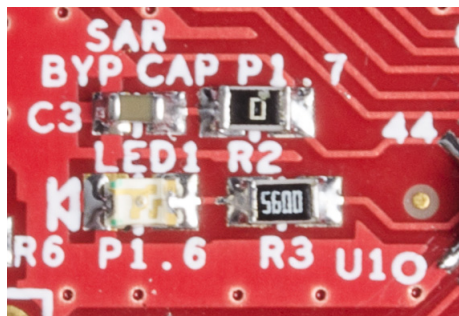
Figure 4-12. Power LED Connection
