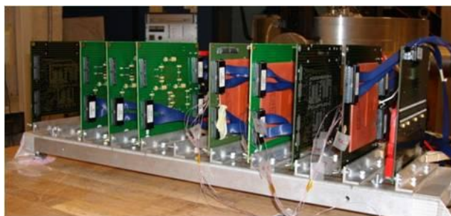
Figure 4. A Photo of the Test Board Sandwiched Between Calibration Boards
