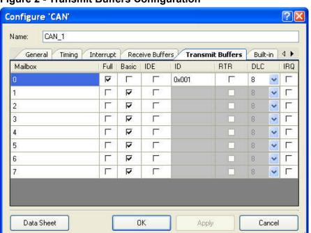
Figure 2 - Transmit Buffers Configuration
