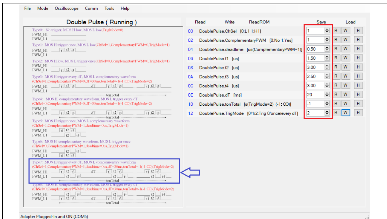
Figure 24 Trigger every mode configuration for the high side MOSFET
