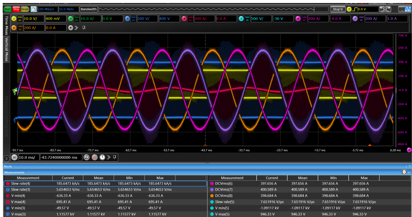
Figure 20 Stationary PWM inverter operation at I_{AC,rms} = 400\ \text{A} and f_{sw} = 15\ \text{kHz}
