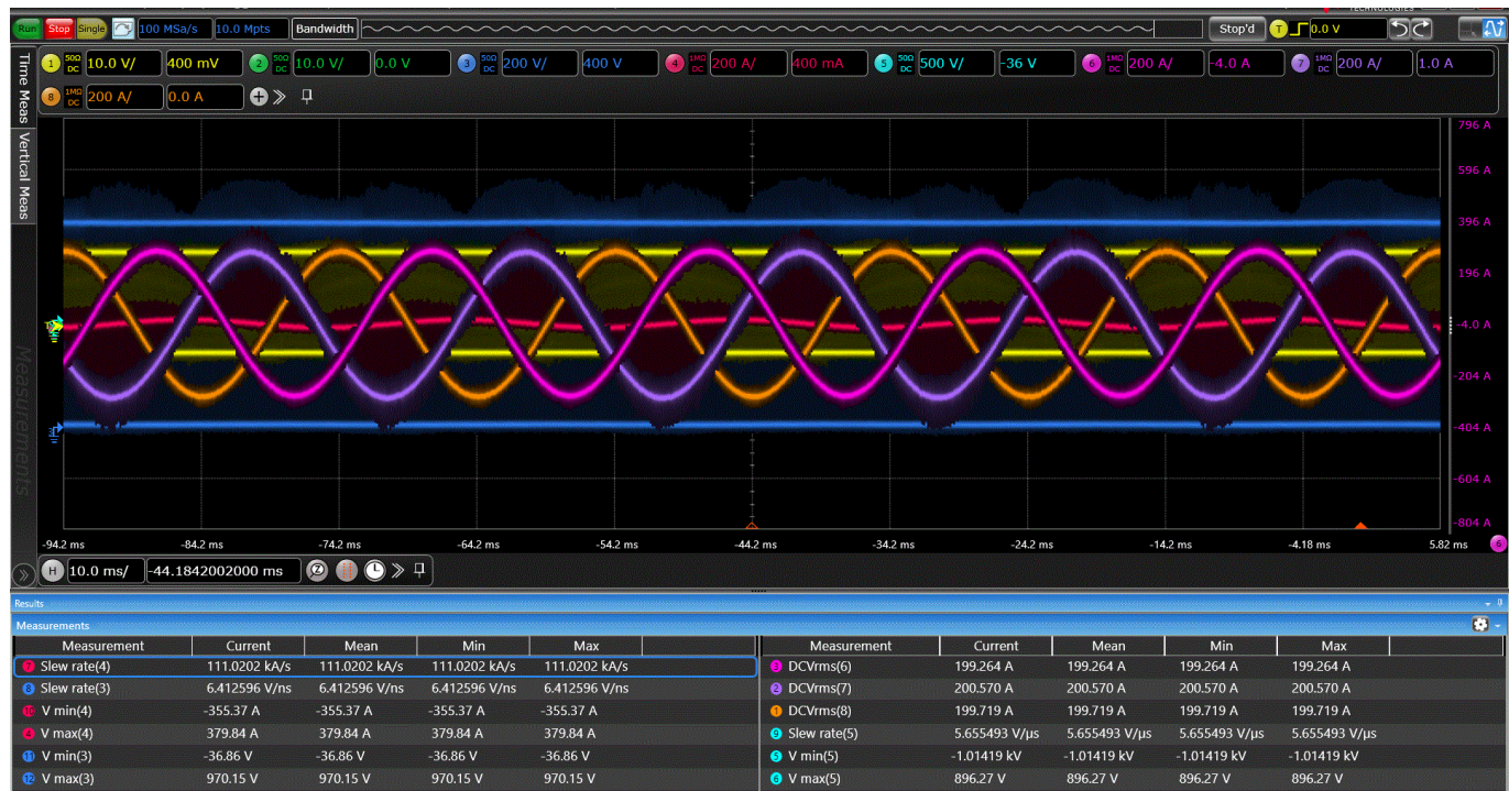
Figure 19 Stationary PWM inverter operation at I_{AC,rms} = 200\ \text{A} and f_{sw} = 15\ \text{kHz}
