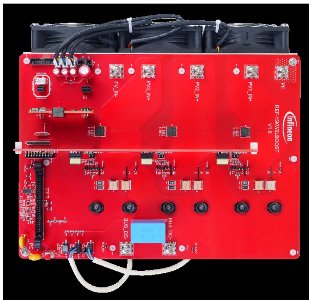
Figure 4 Main power conversion board: REF-15KW2LB00ST
