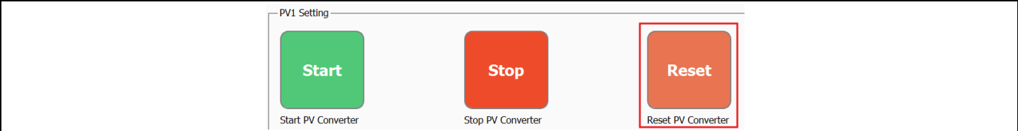
Figure 68 Reset the PV converter
