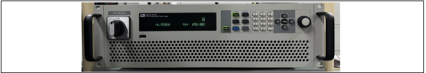
Figure 72 DC source for constant V_{out} in IT6018C-1500-40
