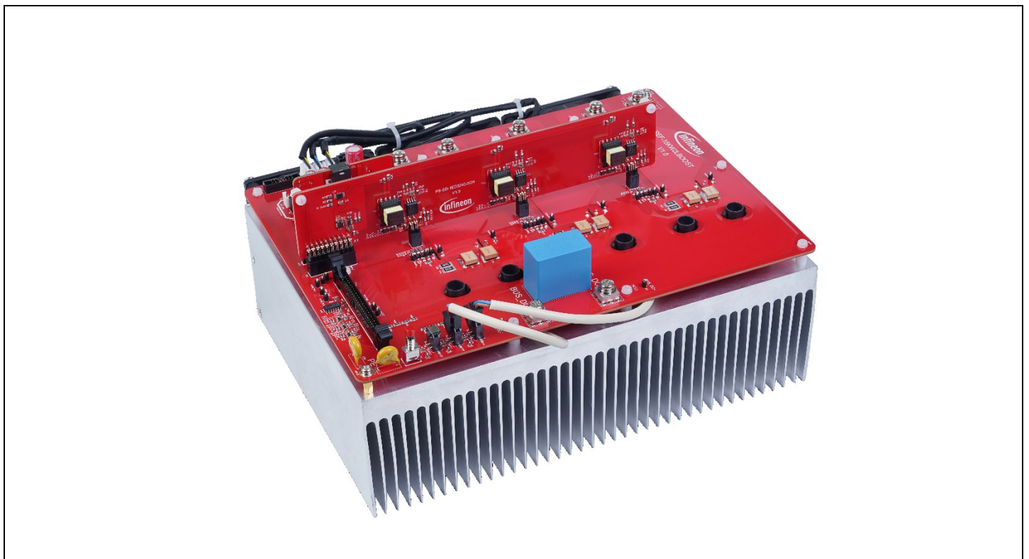
Figure 1 Power conversion board REF-15KW2LBOOST
