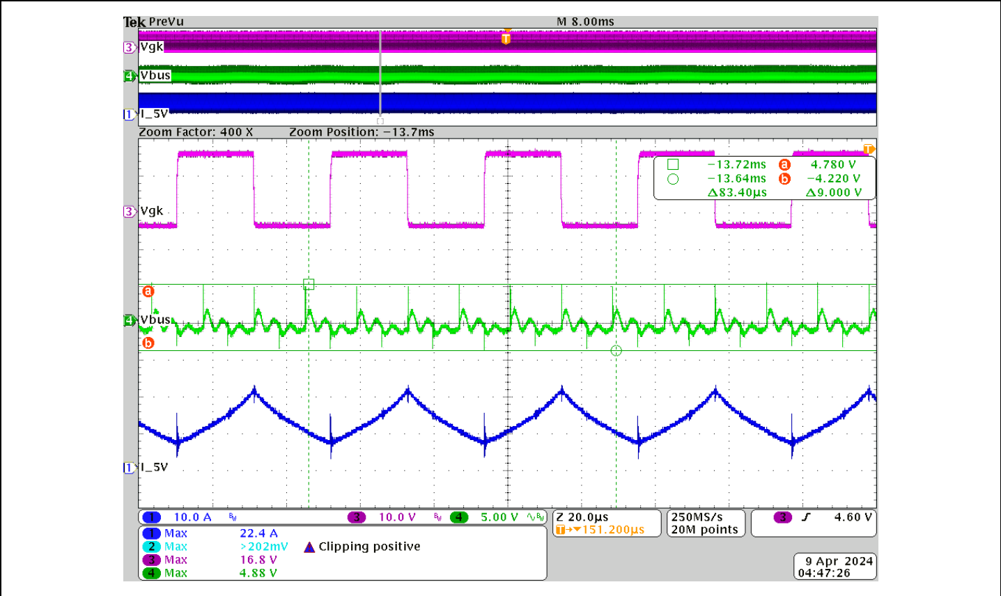
Figure 88 DC-link voltage ripple
