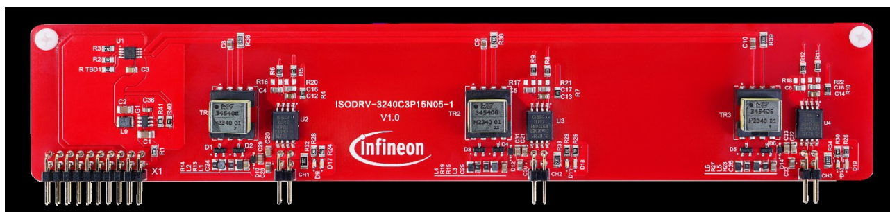
Figure 5 Gate driver board: ISODRV-3240C3P15N05-1
