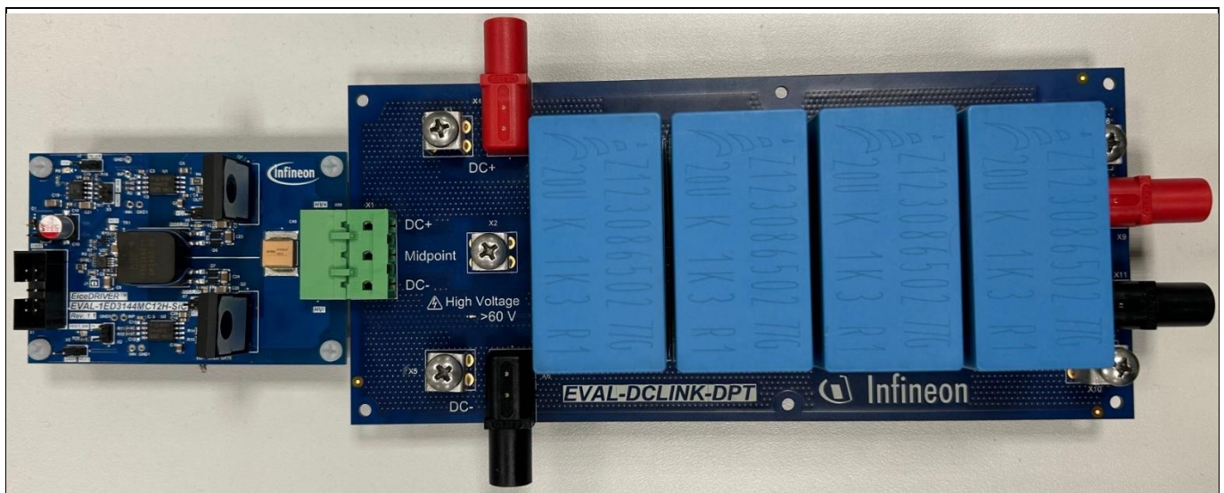
Figure 3 EVAL-DCLINK-DPT connection with double pulse DUT board EVAL-1ED3144MC12H-SiC
