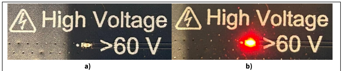
Figure 4 LED status a) safe to handle and b) DANGER High Voltage present
