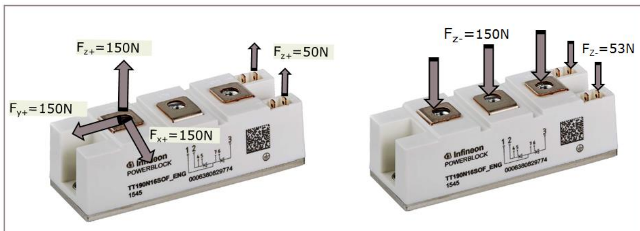
Figure 12.2: Maximum permissible forces during assembly (SB34)
