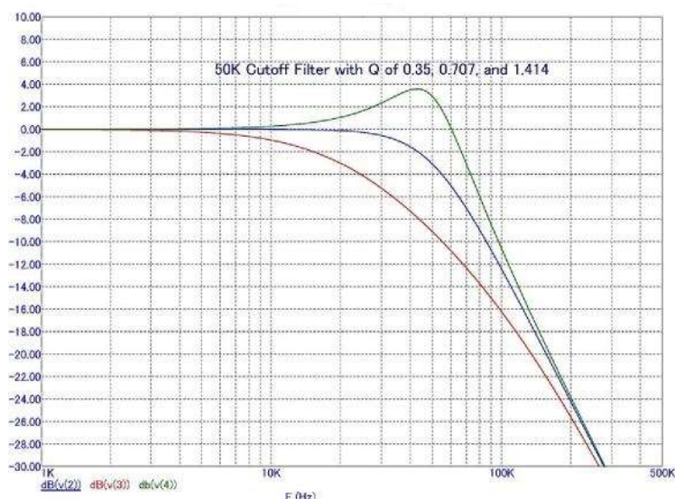
Figure 2 FREQUENCY RESPONSE VS Q OF THE LC OUTPUT FILTER
