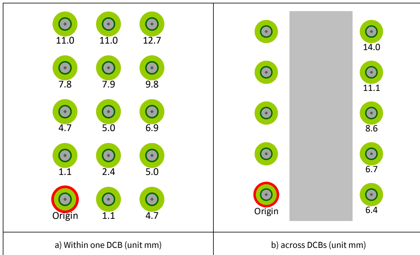
Figure 36 Pin-to-pin creepage distance for high current pin in Easy3B/4B
