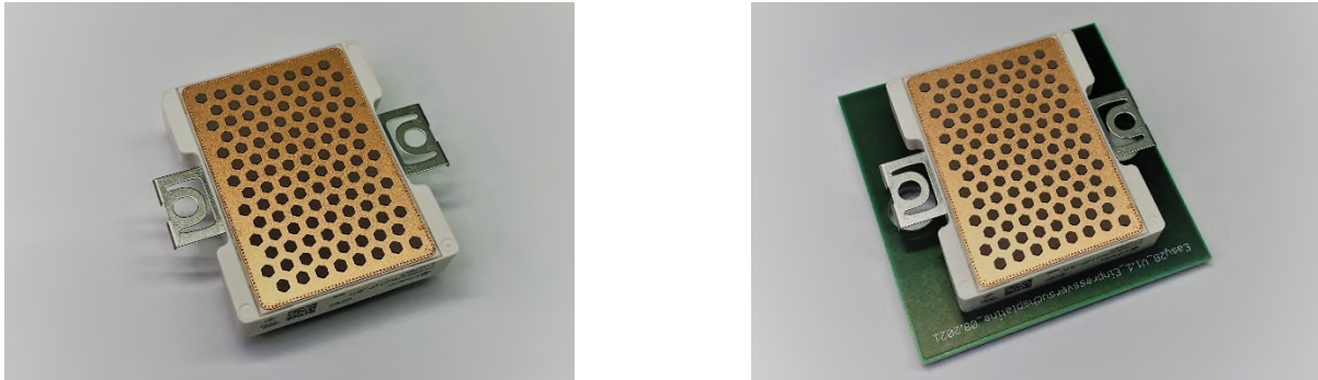
Figure 10 Easy2B with TIM before (shown left) and after (shown right) the press-in process
