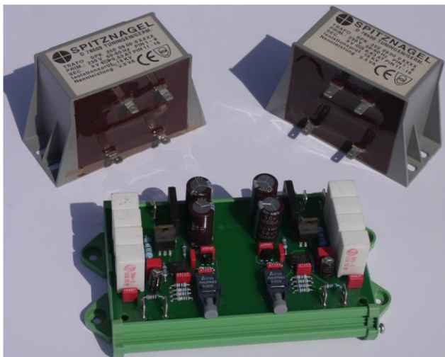
Figure 36. Trigger circuit 2xZB1-10-6600-LWL
