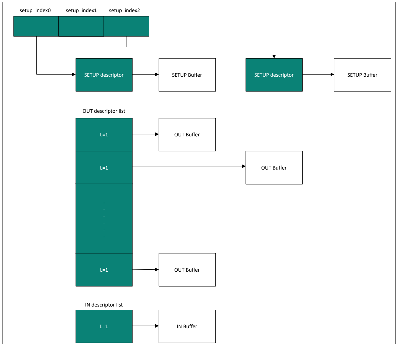
Figure 349 Descriptor lists for handling control transfers
