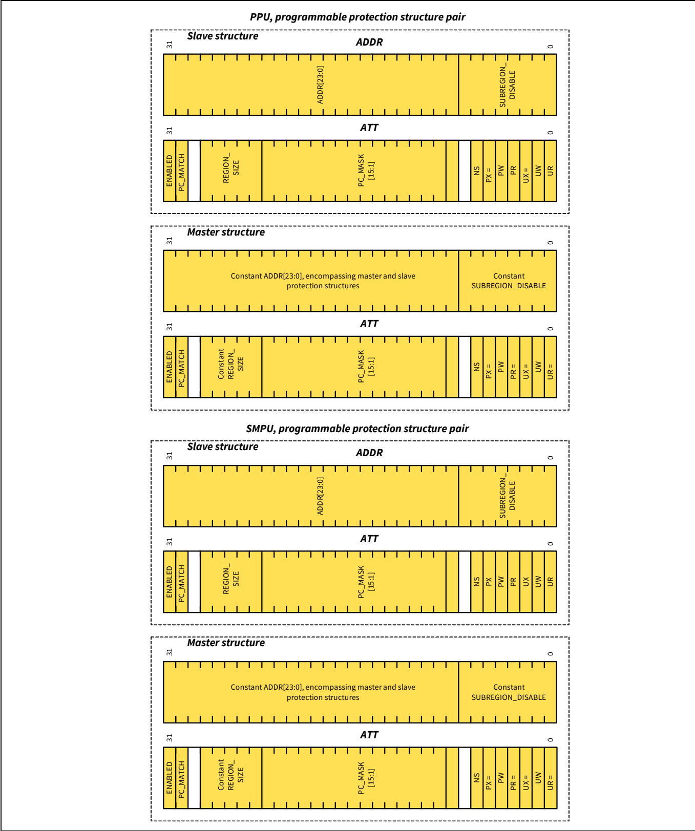
Figure 9-7. Programmable protection structure pair
