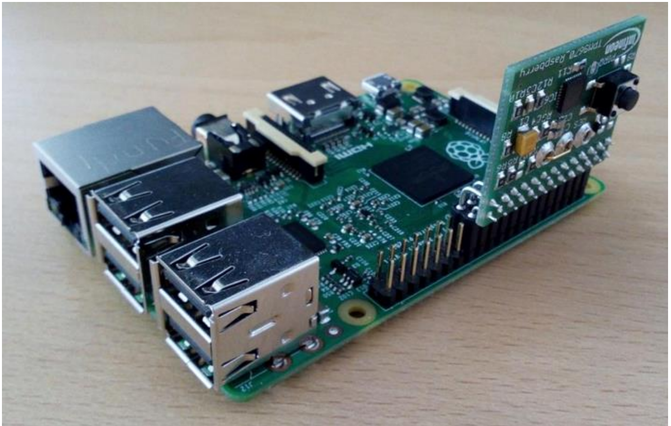
Figure 7 Board connection Iridium - SPI TPM board on a Raspberry Pi® 3
