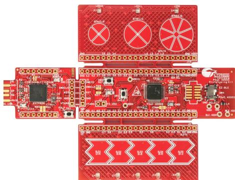
This low-cost kit features a full-featured programmer debugger with a PSoC 4000S device and two snap-away boards enabled for mutual and self-capacitance CapSense designs.
