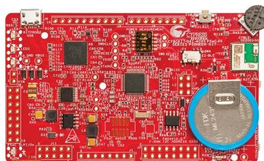
This kit features a PSoC 4000S device with a CapSense trackpad, buttons, and a proximity loop. The board includes an on-board 1Mbit F-RAM, an EZ-BLE™ PRoCTM module, and a rechargeable coin-cell battery.
