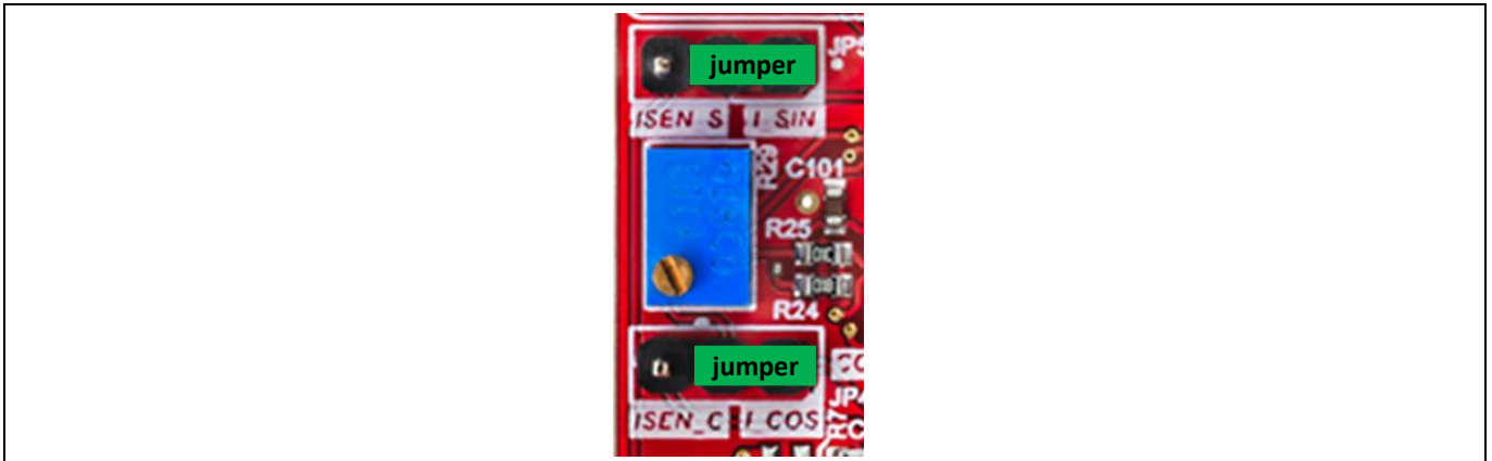
Figure 8 Jumper setting: Connect to I_SIN and I_COS
