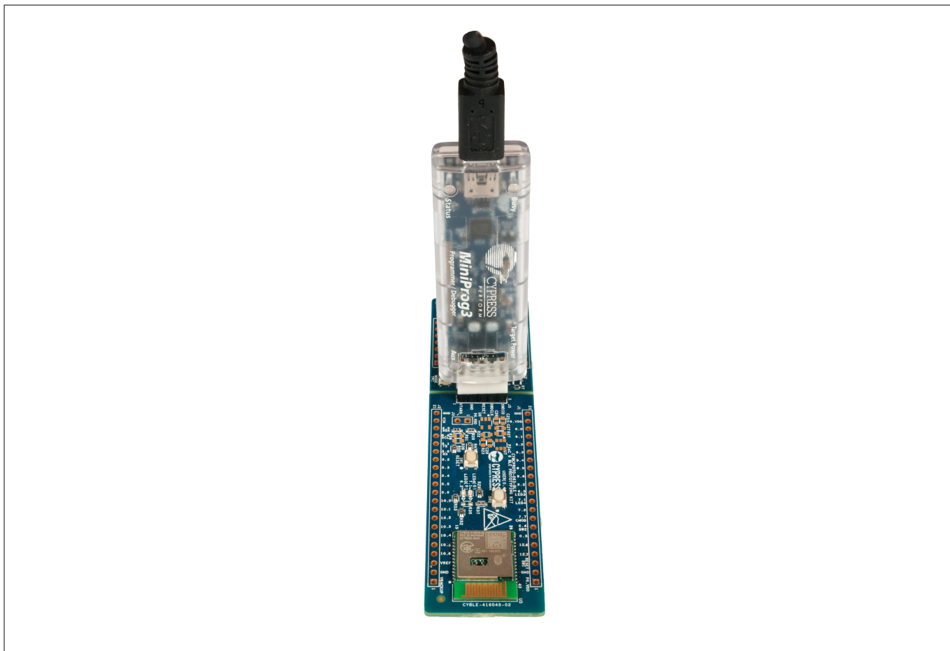
Figure 26 Connecting the CY8CPROTO-063-BLE to a MiniProg4
